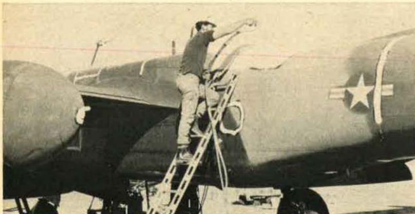
A basic coat of preservative is applied to the fuselage of an A-26 being prepared for extended storage. Eighteen separate operations are undertaken to ensure a thorough job in preparing aircraft for retirement. The dry desert air is an important factor in keeping the stored planes in a condition from which they could be returned to active duty if needed.
