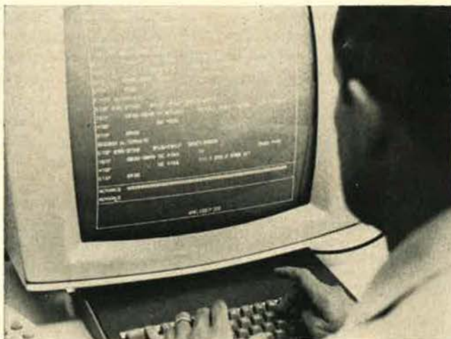
In the new automatic system, frag order preparation is conducted at an electronic display that allows access to large information-storage banks. After preparation, the order is put in the computer for transmittal to the field.
