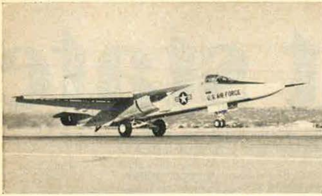
An investigation into the crash of an F-111 in December near Nellis AFB, Nev., which brought about the grounding of all F-111s, has turned up the primary cause of the accident, the Air Force said. It was "structural failure of the left wing" from a "preexisting defect in the steel used in a pivot fitting where the wing joins the fuselage."
