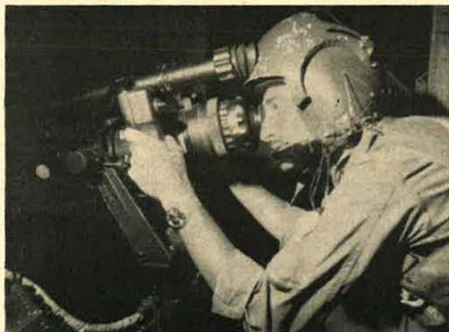
1st Lt. William C. Sawson, from Avenel, N.J., operates an AC-119's night observation scope that uses available light to single out targets for the gunship's awesome weapons.
