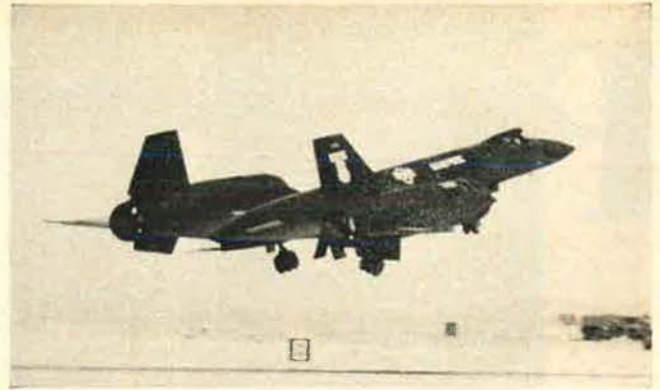
Just a few feet off the ground and the YF-12A already has begun to retract its landing gear during a takeoff. The Mach 3-plus aircraft is one of two that NASA and the Air Force are using at Edwards AFB, Calif., in evaluation flights. The trials among other things, are to provide data for such projects as development of the B-1 bomber.
