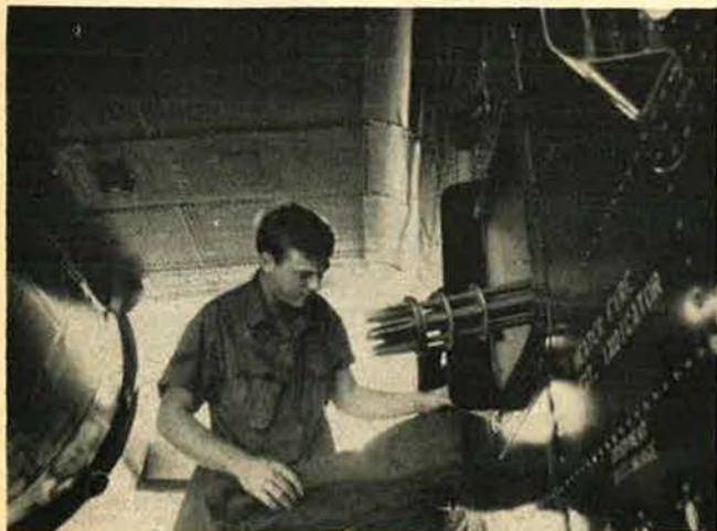
The canvas covering of a Minigun is removed by A1C Edwin Bryant of Waynetown, Ind. An AC-119 Shadow gunship's four Miniguns can be fired individually or in unison.
