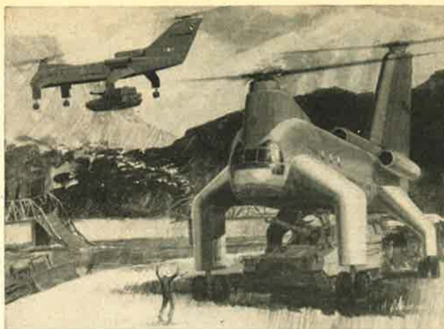
An artist's concept of the mammoth and grotesque heavy lift helicopter the US Army has its sights on. If the money is forthcoming, prototypes could be ready by 1976. Design specs call for the big bird to have a lift capability of twenty-three tons at 4,000-foot altitudes, even in warm weather.
