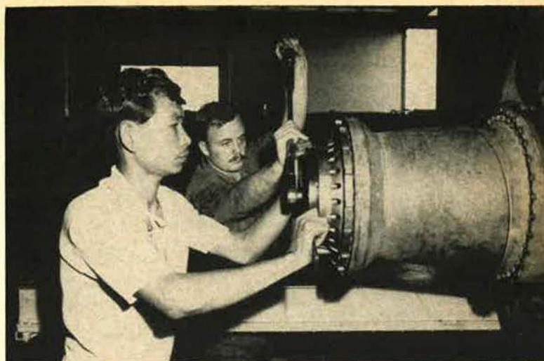
Sgt. David A. Johnson with the 355th Field Maintenance Squadron's propulsion branch and Prayoon Suwanjack, one of fifteen Thai employees at the propulsion branch at Takhli RTAFB, torque the number-four bearing on a J75 engine.
