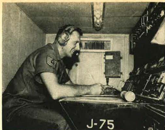
Monitoring the control panel of a J75 engine test cell is TSgt. Phillip Stratford. Performance procedure requires that following maintenance the jet engines undergo static tests before they are reinstalled in the aircraft.
