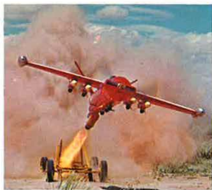
A Jato rocket boosts the Cardinal from a simple zero-length launcher. Made flight-ready in minutes, checked out and started in seconds, it can be launched with a 20 knot tail wind.
