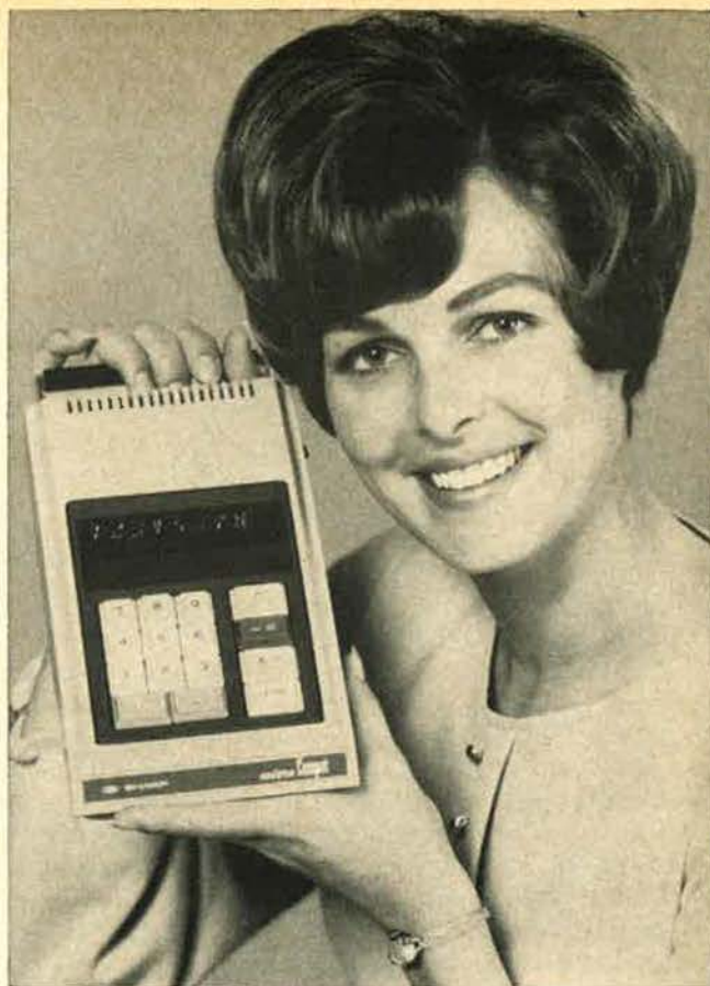
Hayakawa Electric Company in Japan builds the desk-top calculator above, using three large-scale integrated (LSI) microelectronic circuits that it imports from Autonetics in the United States. Autonetics is supplying large numbers of these LSI chips under the terms of a $30 million contract.
