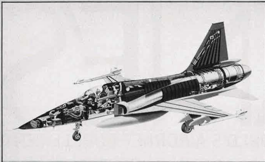
Cutaway emphasises the use made of every cubic inch of the F-5G's minimal space
