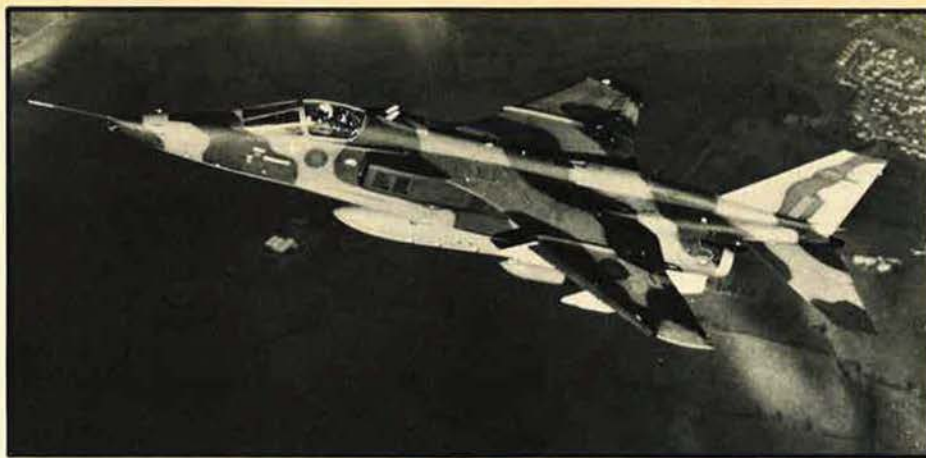
The Anglo-French-developed Jaguar is a close-support and tactical-strike aircraft that doubles as an advanced and operational trainer.
