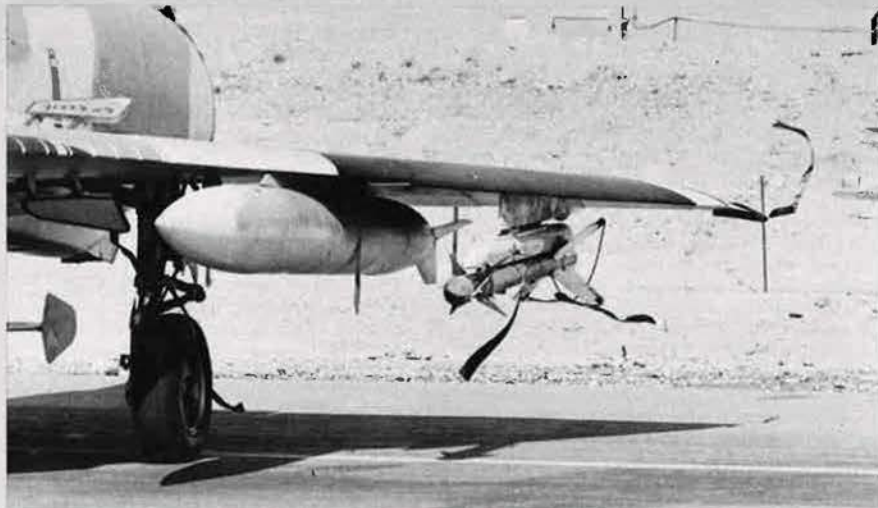
Sidewinder missile on a Kfir-C2 at its operational base 'somewhere in Israel'
