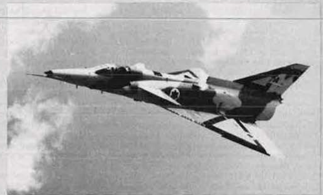
The Kfir-C2's canard foreplanes are shown clearly in this air-to-air shot
