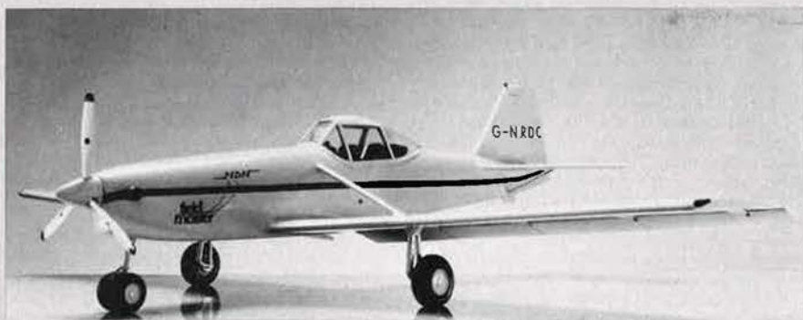
Model of NDN 6 Fieldmaster agricultural aircraft. Production version will have a single nosewheel
