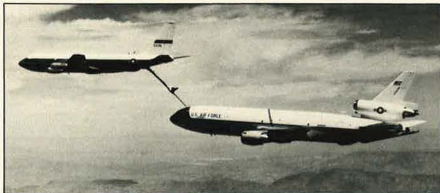
An Air Force KC-135 tanker refuels a McDonnell Douglas/USAF KC-10A advanced tanker/cargo aircraft near the Sierra Nevadas of California during a recent test flight. Boom configuration allows KC-10s to refuel each other, as well.
