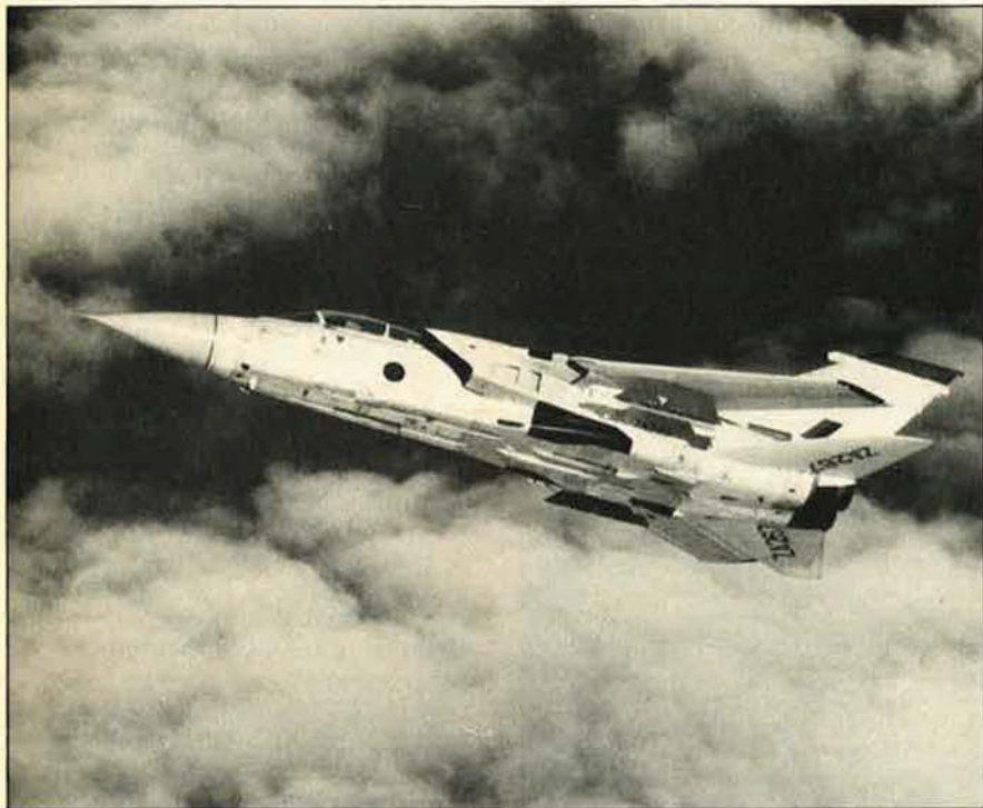
Recent maiden flight of the second of three prototypes of the Tornado Air Defense Variant (ADV), the Royal Air Force's latest long-range interceptor. This particular aircraft will be used for weapon-systems integration and development. The trination swingwing Tornado is capable of speeds in excess of Mach 2 at altitude.
