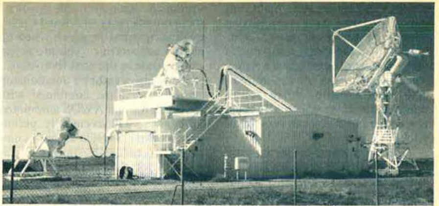
The ANIFRR-95 Radio Solar Telescope System monitors solar activity. Sun bursts can adversely affect HF propagation, satellite systems, and manned space flights.
