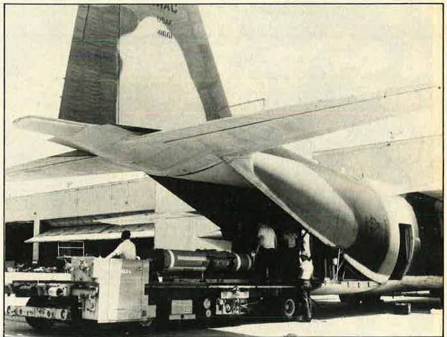
A dummy mine is loaded aboard a USAF C-130 Hercules during a test of a Cargo Aircraft Minelaying System to demonstrate that Air Force transports can supplement the Navy's aerial mine-laying capabilities. Initial gravity drop tests have been conducted at Eglin AFB, Fla. See item beginning on opposite page.
