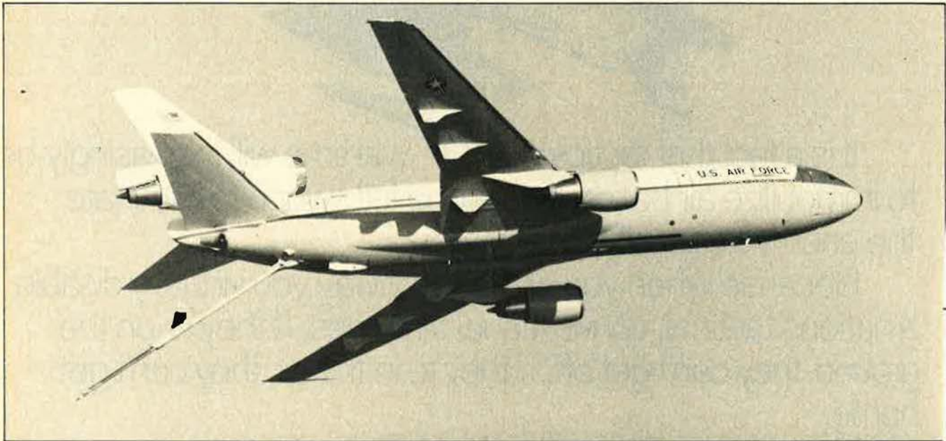
Above, at Edwards AFB, Calif., extension tests of the aerial-refueling boom of USAF's new tanker, the McDonnell Douglas KC-10A. The tail-boom system, operated under digital fly-by-wire control, can deliver 1,500 gallons of fuel per minute to refueling aircraft. Left, a British Army Lynx helicopter launches an antitank TOW missile during a test-firing program. See item.
