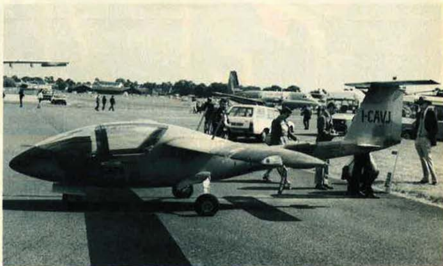
The tiny jet-powered Caproni C22J is Italy's concept for a fuel-efficient primary trainer for the 1980s. (J. M. G. Gradidge)
