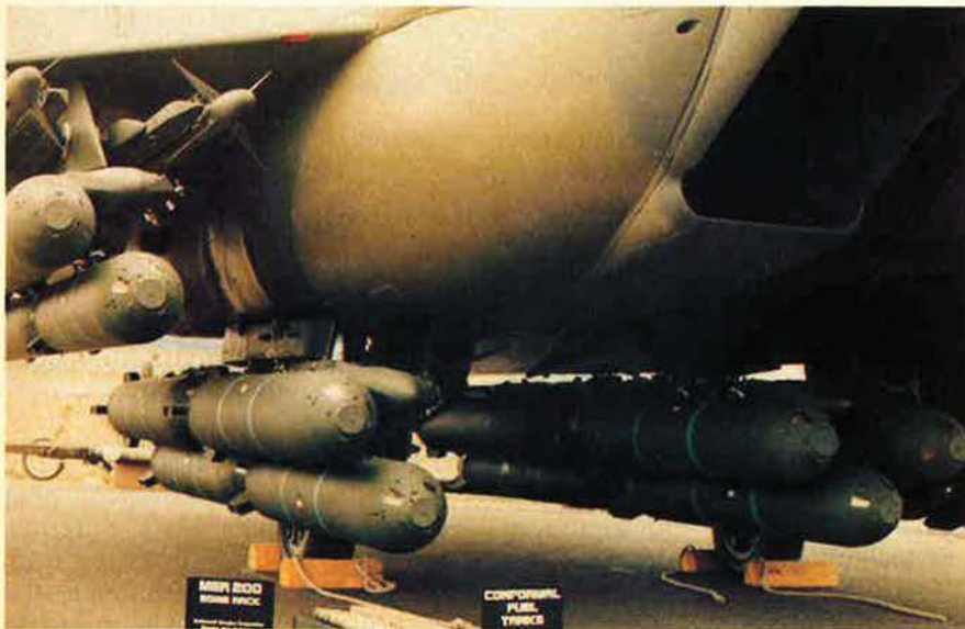
F-15B Strike Eagle closeup shows arrangement of Rockeye bombs and AIM-7 Sparrow missiles grouped around conformal fuel tank.
