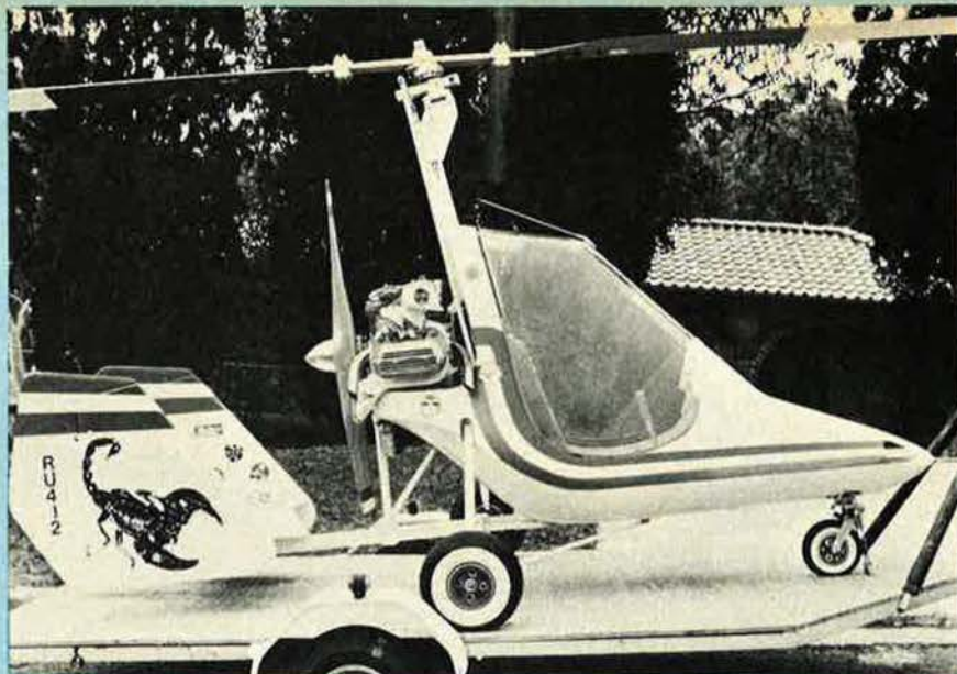
Prototype of the Minty Skyhook single-seat gyroplane, intended for sale in ready-to-fly form
