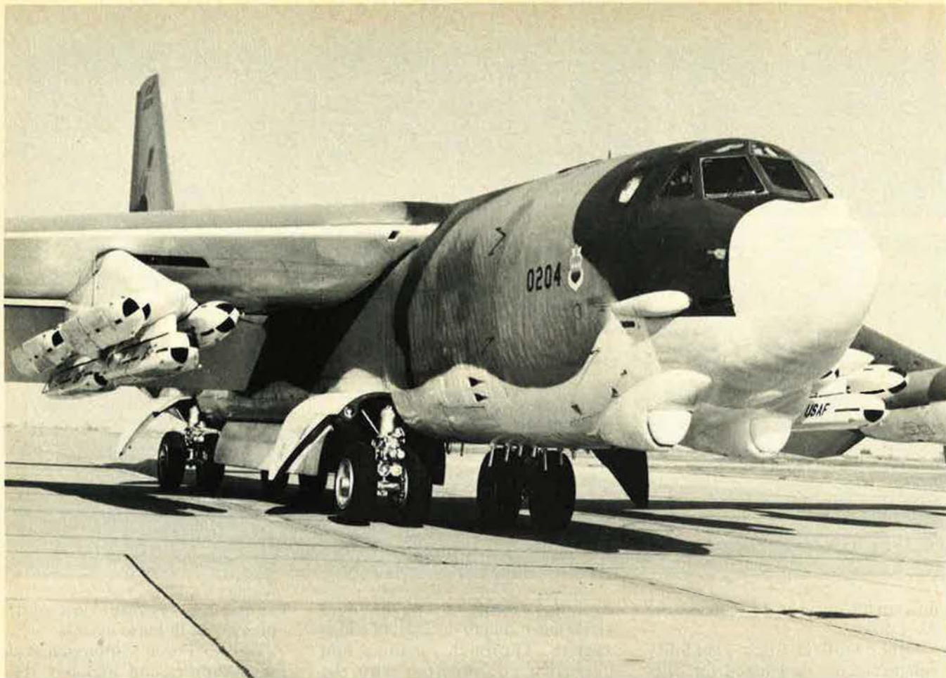
SAC's B-52G is the only manned bomber able to carry the Air-Launched Cruise Missile, twelve externally and eight internally. One ALCM squadron may be operational by 1982.
