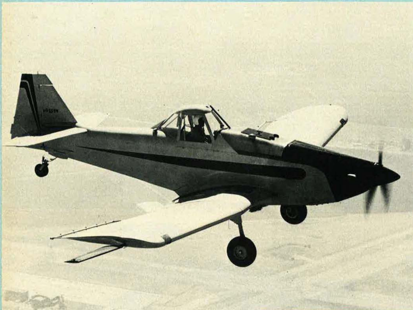
Except for its P&WC PT6A-11AG turboprop, the Model 620TP is generally similar to the piston-engined version
