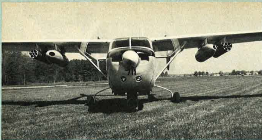
For counter-insurgency operations, the Sentry carries an underwing armament of gun pods and rocket launchers
