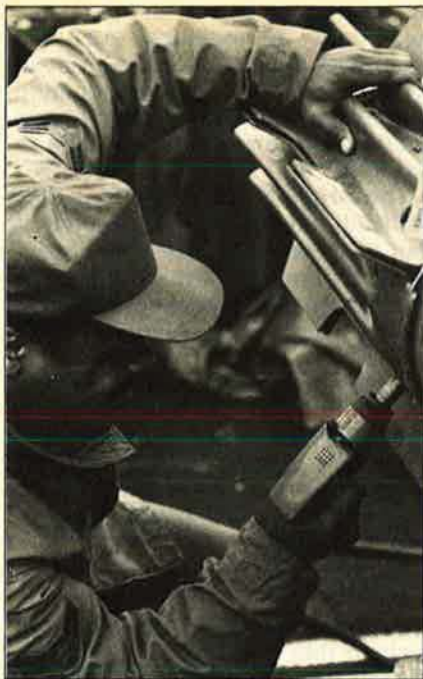
At Spangdahlem AB, Germany, A1C Persel Gilliam sets the screw on a bomb drag fin. During Salty Radome, munitions personnel and augmentees recently conducted the largest conventional munitions buildup exercise in USAFE.
