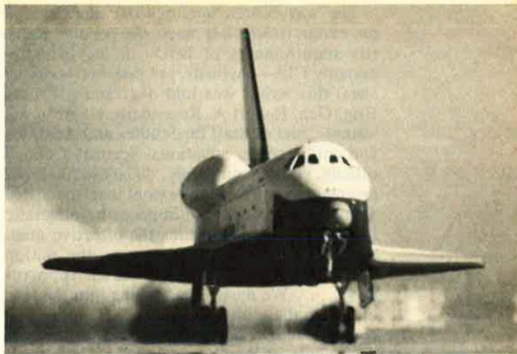
Shuttle Enterprise landing after separation from a 747 over the Mojave Desert and a five and one-half minute free flight.
