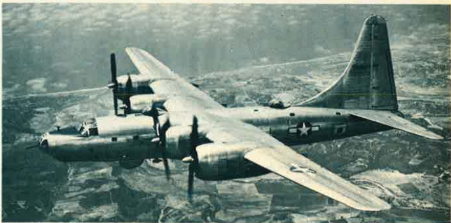
The production version of the B-32 was eighty-two feet one inch long. It had a wingspan of 135 feet and stood thirty-two feet two inches high. Four 2,200-horsepower Wright R-3350-23 engines gave the 100,000-pound aircraft a maximum speed of 357 mph at 30,000 feet. Cruising speed was 290 mph. The Dominator carried a crew of ten, 8,000 pounds of bombs, and 5,460 gallons of fuel.
