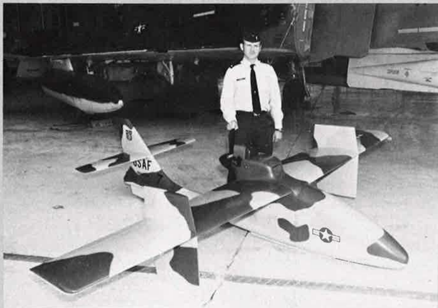
USAF FDL XBQM-106 experimental mini-RPV, with wing side-force panels
