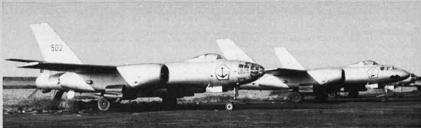
Standard bomber and (behind) tandem-cockpit training versions of the Il-28, in store in Indonesia (K. E. Sissons)
