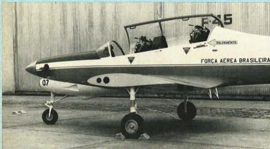
Wooden mockup of the EMBRAER EMB-312, under development as the Brazilian Air Force's new T-27 basic trainer
