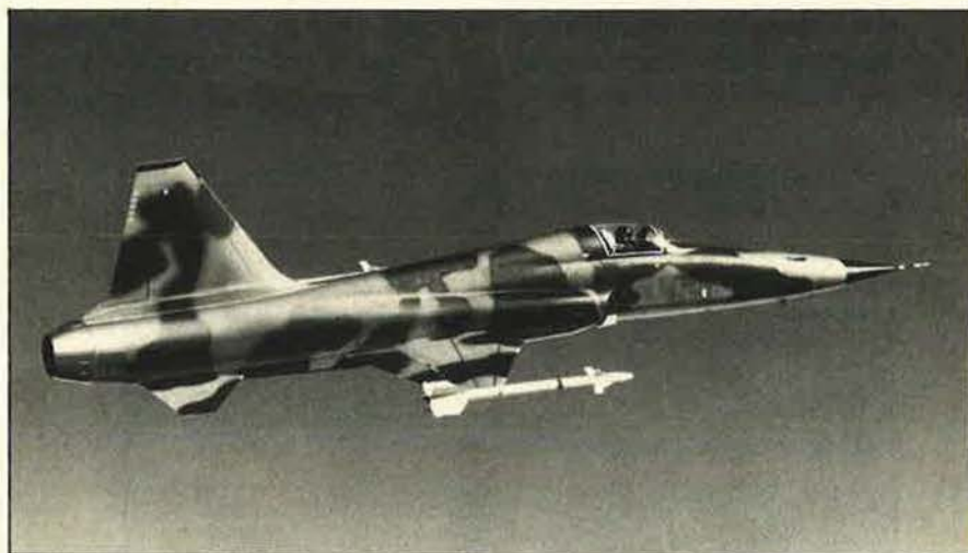
An artist's concept of Northrop Corp.'s F-5G, the single-engine version of the highly successful tactical F-5 being specifically designed as a new intermediate export fighter. Because of the G's commonality with other F-5 versions, Northrop anticipates a significant international sales potential for the aircraft, to be powered by a GE F404 in the 16,000-lb.-thrust class.
