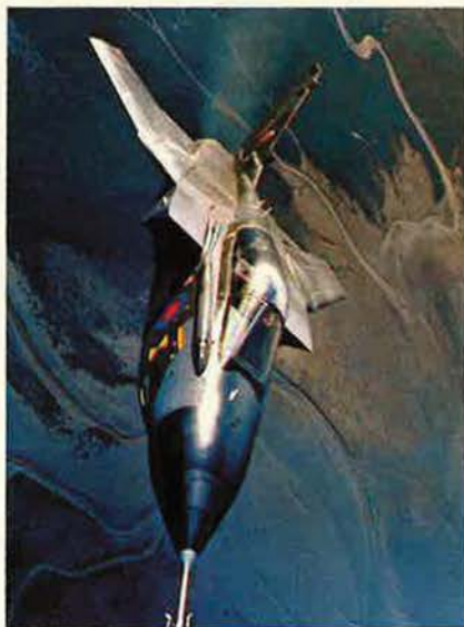
There is no trim change and little change in handling with the wings in the fully swept position. (Crown Copyright)
