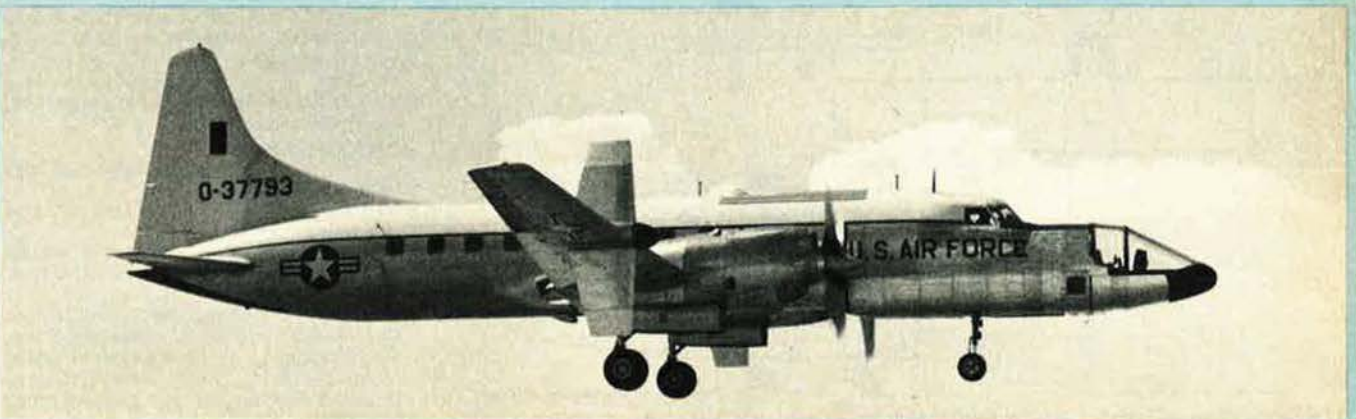
Calspan's Total In-Flight Simulator, an extensively modified Convair/USAF NC-131H
