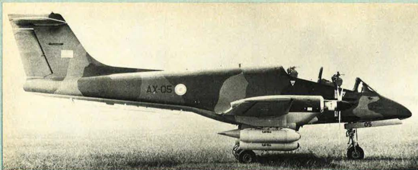
This view of the Pucara Bravo shows clearly the deepened front fuselage, housing larger guns
