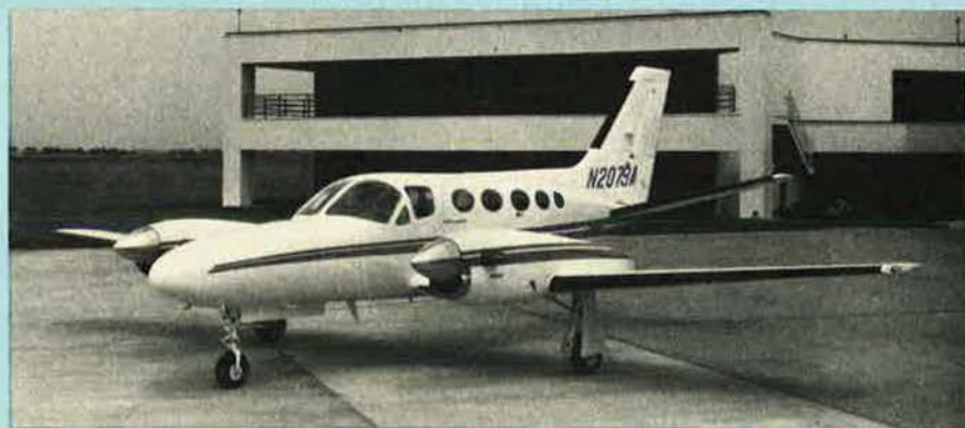
The new Cessna Model 425 Corsair, a turboprop development of the piston-engined Model 421 Golden Eagle
