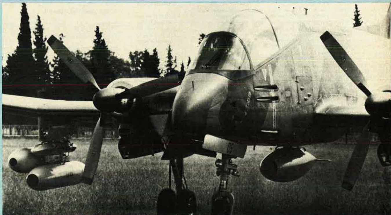
Prototype of the IA 58B Pucará Bravo counter-insurgency combat aircraft, showing underwing and underbelly stores
