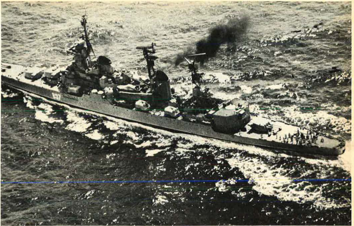
The Zhdanov, part of the Soviet Black Sea Fleet, is one of two Sverdlov-class cruisers converted during the 1970s to a flagship configuration, including extensive C 3 facilities and accommodations for an admiral and his staff. Note the extensive
