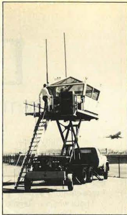
The self-contained, mobile air traffic control tower developed by Lockheed Aircraft Service Co. contains all equipment needed for VFR control over aircraft within a designated zone.
