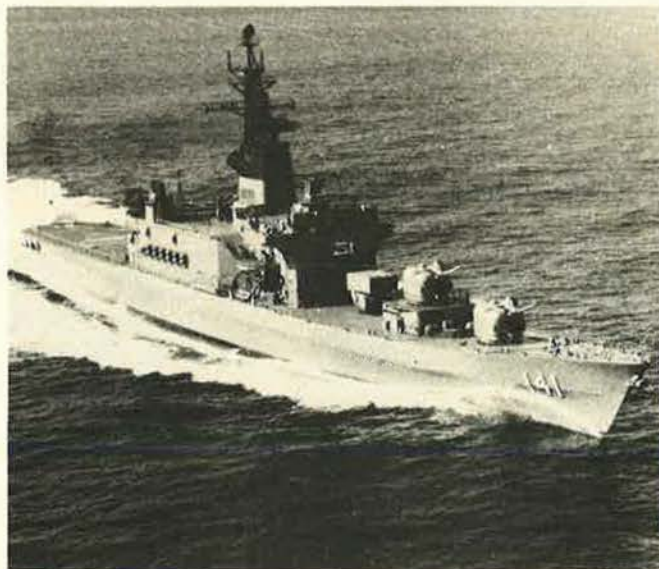
Two ships of the Haruna class helicopter destroyer have been commissioned, and construction continues on two more. Maximum speed is thirty-two knots. Armament consists of three antisubmarine helicopters, two five-inch rapid-fire guns, one ASROC unit, and two triple-mounted, short-range torpedo tubes.
