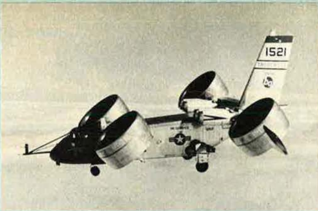
Bell/Navy X-22A V/STOL research aircraft, used by Calspan to investigate advanced control systems for deck-landing helicopters
