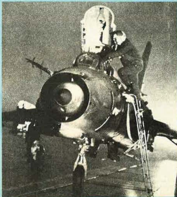
Close-up of the nose of a 'Fitter-D' model of the Sukhoi Su-17, showing clearly for the first time the undernose radome and the laser marked target seeker in the undersurface of the intake centrefield
