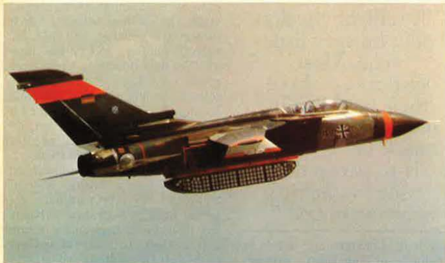
A Luftwaffe Tornado with the MW-1 cluster dispenser that ejects a large number of small munitions to either side of the aircraft.
