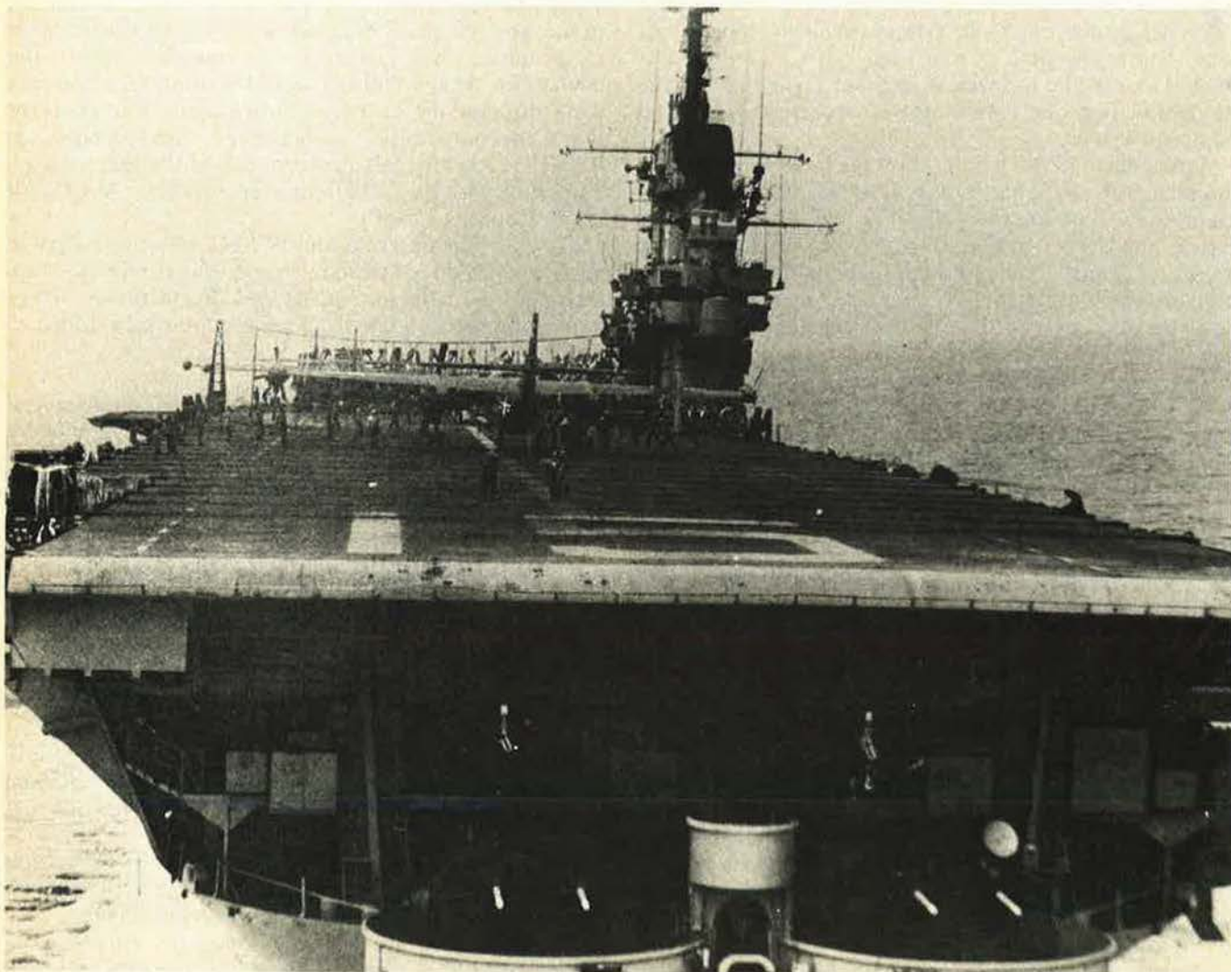
This is what an incoming pilot saw just before landing on one of the old straight-deck carriers. The heavy attack AJ Savage that had just landed would, of course, have been cleared from the landing area. Note the arresting cables on the deck.
