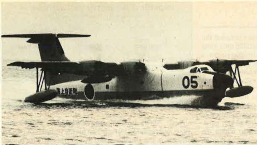
The PS-1 antisubmarine flying boat, of Japanese design and manufacture, is capable of takeoffs and landings in rough seas with wave heights up to three meters. External armament includes launchers beneath each wingtip for air-to-surface rockets, and underwing pods for torpedoes. It carries a crew of twelve and has an operational range of about 2,400 nautical miles.
