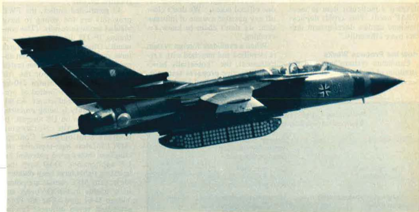
The MW-1 cluster munitions dispenser on Luftwaffe Tornado aircraft is the principal example of current applications of the twelve-year-old TREBO technology program.
