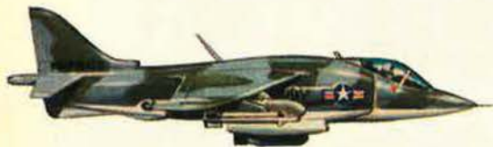
Harrier – the world's first operational V/STOL combat aircraft.
