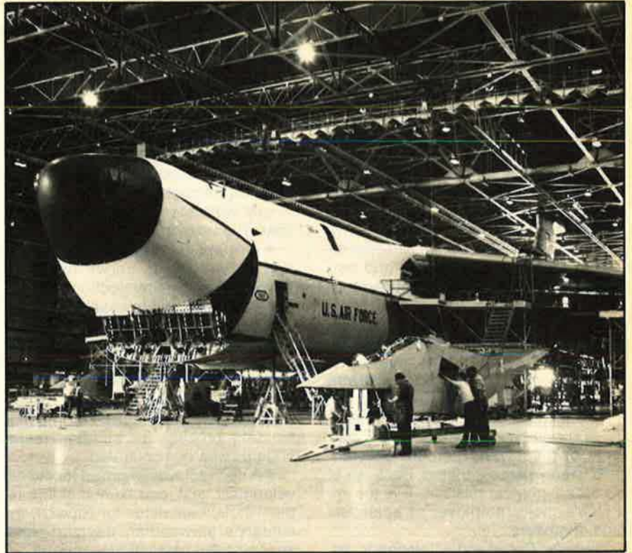
USAF C-5 Galaxy goes through a phase of depot-level maintenance inside the huge Aircraft Maintenance Hangar at AFLC's San Antonio Air Logistics Center at Kelly AFB, Tex. Kelly AFB is the only USAF installation overhauling the giant cargo carrier.
