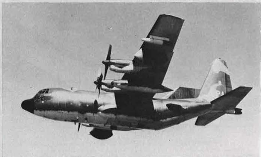
Lockheed EC-130E electronic surveillance version of the Hercules, which has replaced the Lockheed EC-121
