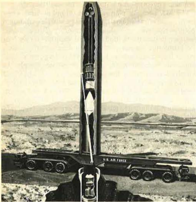
Of the three MX/MPS deployment modes, the vertical shelter, shown here, is the least expensive, but also the least well adapted to rapid reconfiguration in a crisis, or on tactical warning of an attack.
