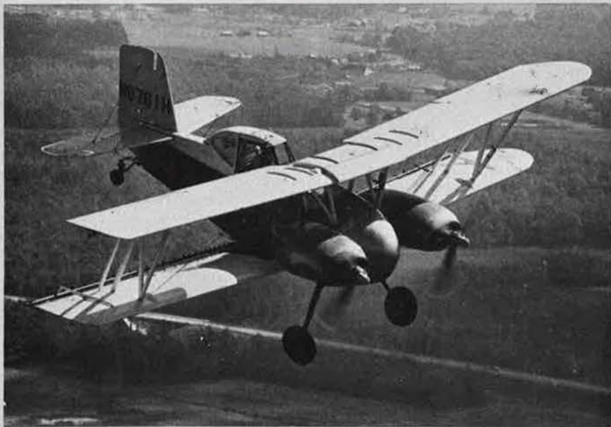
Twin Cat agricultural aircraft, a twin-engined conversion of the well-known Grumman/Gulfstream American Ag-Cat (Howard Levy)
