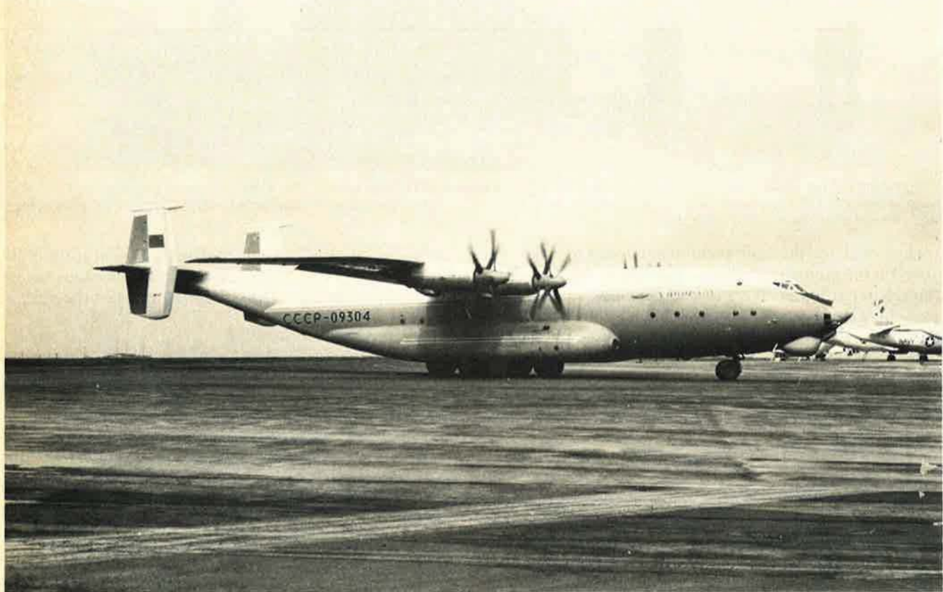
Above: The Antonov An-22 turboprop-powered long-range cargo aircraft is fitted with dual counterrotating propellers for each of its four engines. It is the largest Soviet strategic airlifter, and has been used extensively in flights to the Western Hemisphere and Africa, as well as the December 1979 invasion of Afghanistan. At right: Close-up of navigator's station on the Antonov An-22 cargo transport. The aircraft's unique dual counterrotating propellers can be seen to right of the nose.
