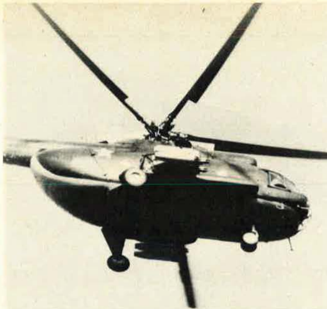
The Mi-8 Hip helicopter is a standard utility helicopter that has evolved into a gunship as well. It has been exported to at least nineteen countries outside the Soviet Union. This version has three stores pods on each side of the fuselage. An Mi-8 commercial version is in use by Aeroflot.
