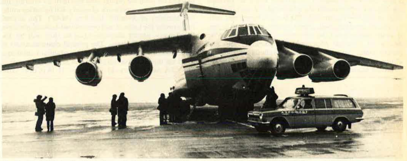
The Ilyushin Il-76 is the Soviet counterpart to the USAF C-141. It has a payload similar to the C-141's, but is capable of operating from more austere airfields. Current production is three per month, with several hundred contemplated for purchase by the Soviet Air Transport Force and an additional one hundred for Aeroflot.
