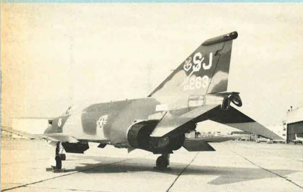
APR-38 antennae in a rear-facing fin-tip pod help to distinguish the F-4G
