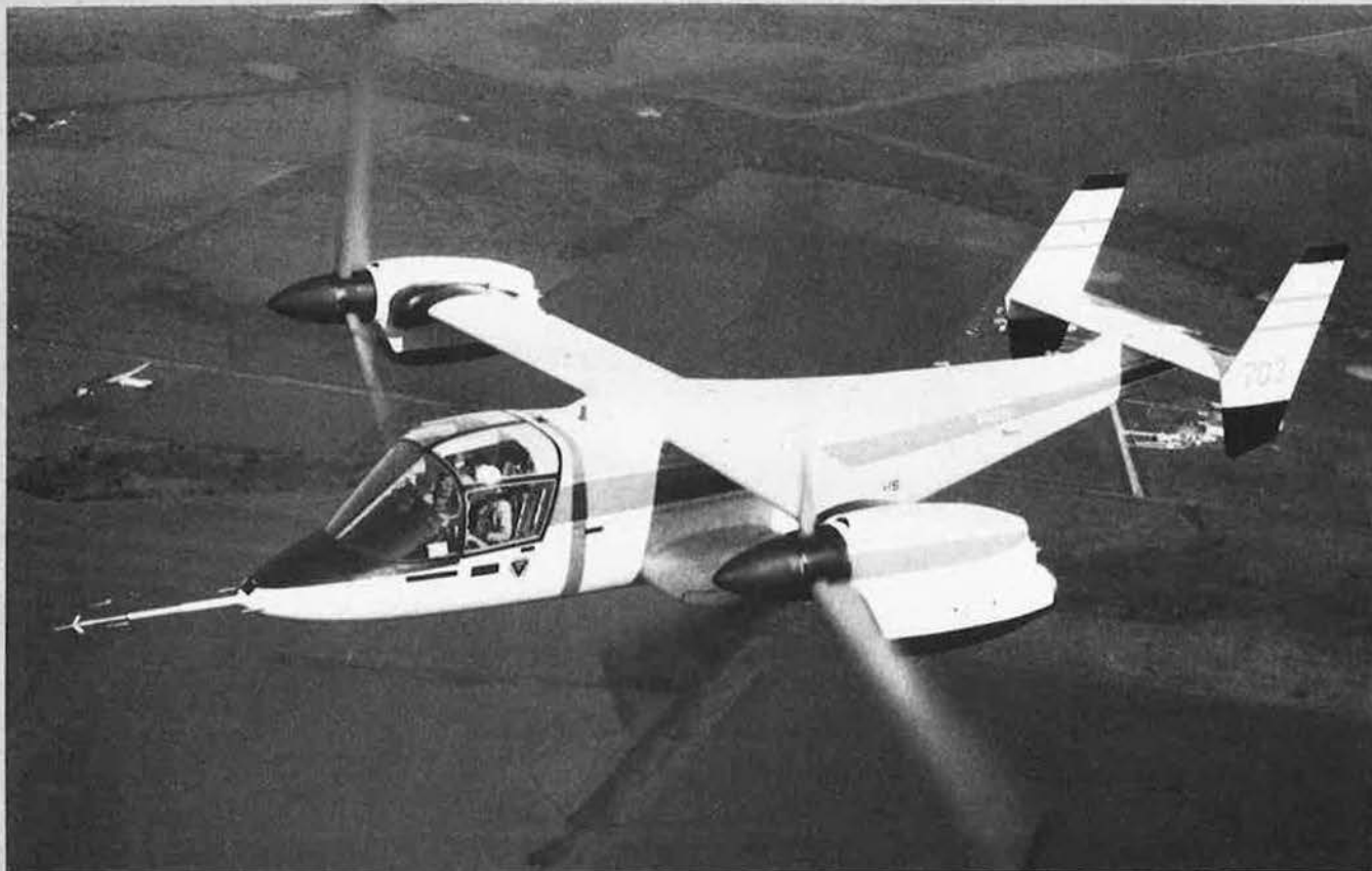
Second prototype of the Bell XV-15 tilt-rotor research aircraft in conventional aeroplane cruising configuration
