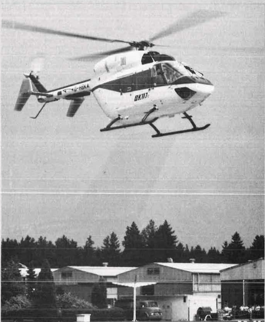
Prototype of the MBB/Kawasaki BK 117 twin-turbine multi-purpose helicopter
