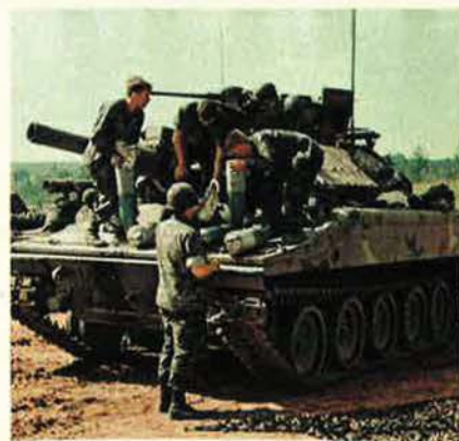
Loading ammunition aboard the tracked and air-droppable Sheridan armored reconnaissance vehicle.
