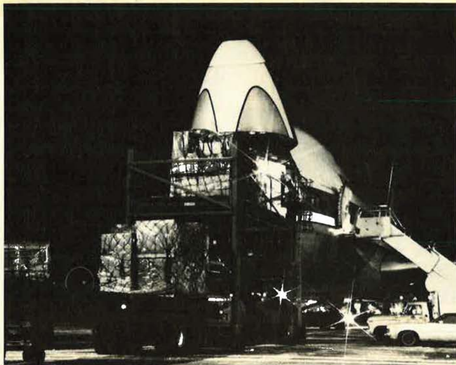
Palletized cargo is loaded straight into the main cargo deck of this Pan American 747 freighter. Seventy-six Pan Am planes are in CRAF.
