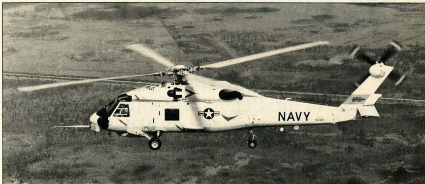
The first prototype of the advanced technology SH-60B Seahawk helicopter Sikorsky Aircraft is developing for the US Navy made its maiden flight in mid-December at the company's flight center in West Palm Beach, Fla. Seahawk is to serve as air vehicle in the Light Airborne Multi-Purpose System (LAMPS), designed to seek and destroy enemy subs and ships.
