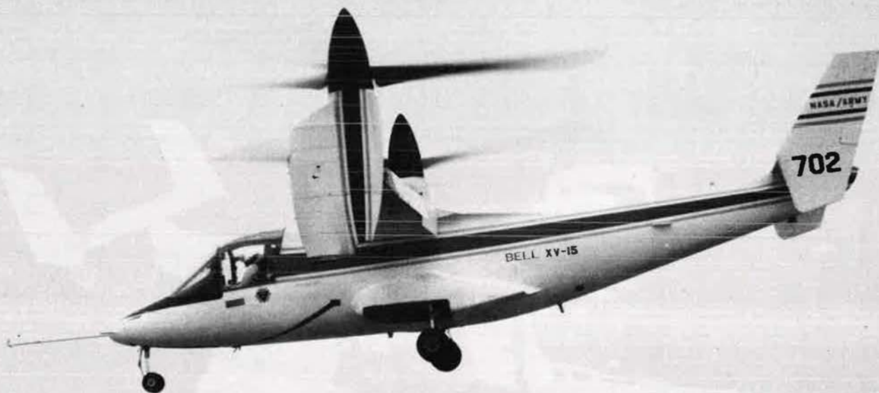
First prototype of the Bell XV-15 in hovering mode, with wingtip pods tilted vertically
