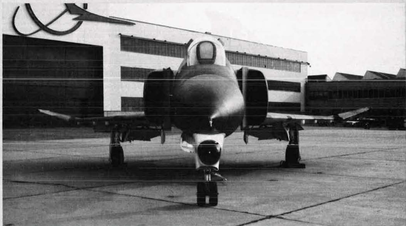
The laminated glassfibre chin pod replacing the original gun fairing is seen clearly in this head-on view of the F-4G Advanced Wild Weasel
