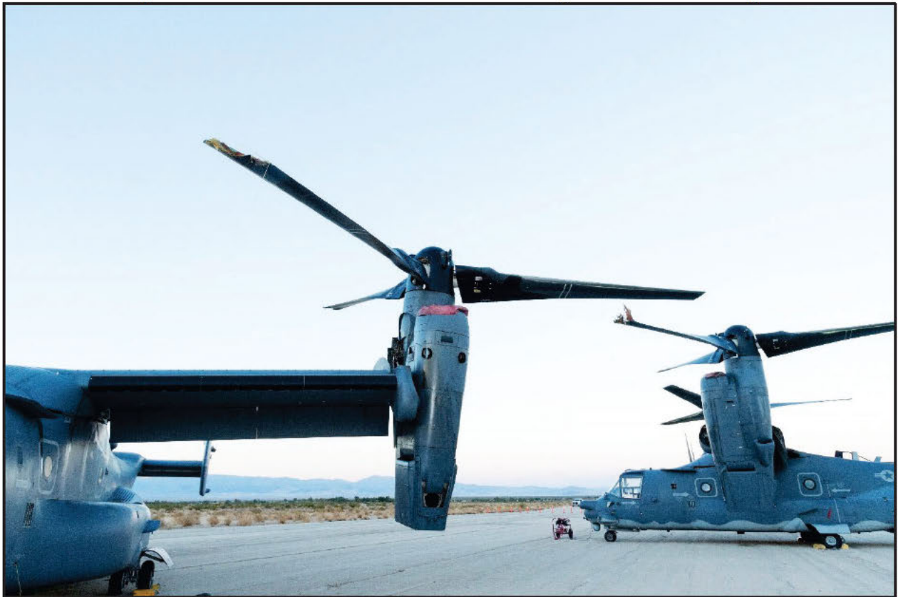
Figure 7.0 – MA's and Parked Aircraft's Proprotor Blade Damage
