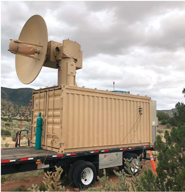
The Air Force Research Laboratory's Tactical High-Power Operational Responder (THOR) employs microwave energy to defeat multiple, concurrent targets, such as drone swarms.
