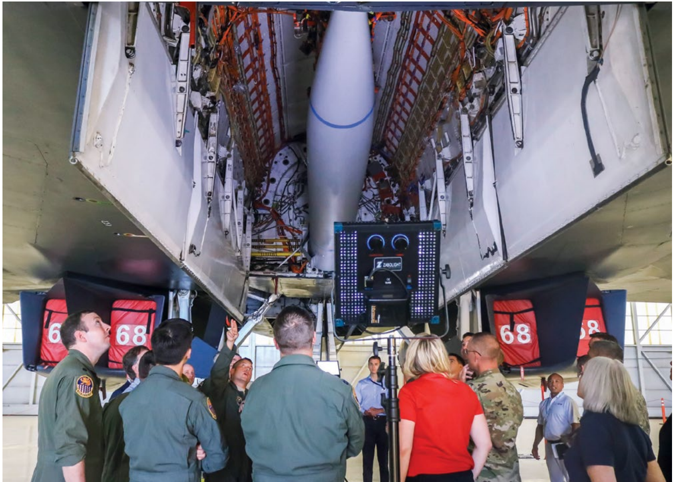
Bomb bay modifications allow the B-1 to accommodate 5,000-lb munitions and, potentially, hypersonic weapons. Lt. Col. Dominic Ross, B-1B program element monitor for Air Force Global Strike Command, explains the modifications to visitors.
