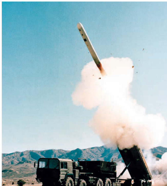
A ground-launched cruise missile emerges from the transporter-erector launcher during a test firing at the Utah Test and Training Range in 1982. GLCMs were deployed to Belgium, Britain, Germany, Italy, and the Netherlands.
