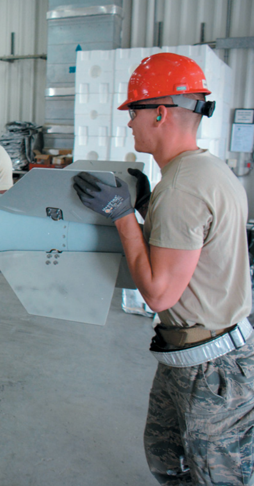
SrA. Christopher Haynesworth, left, and SSgt. Daniel Eisenhart install a tail kit on a JDAM at Al Udeid AB, Qatar. Precise attacks on even a relatively low-level tactical target impose costs on adversaries; they know USAF has the capability to do it at any time.
