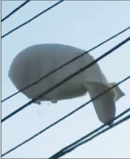
The damaged aerostat slowly sinks to the ground. The Puma's pilot, seeking to avoid footballers playing on the soccer field landing zone, hit the cable that tethered this reconnaissance balloon to the ground. The cables were designed to snap if a rotor blade hit them—but it didn't happen this time.
