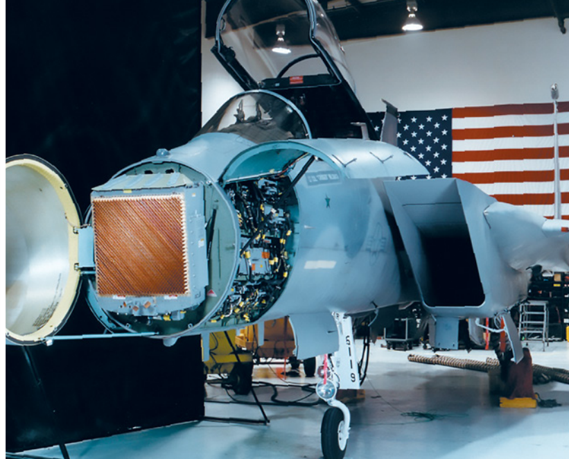
Version 2 of the active electronically scanned array, or v2 AESA, on an F-15. Eagles are getting the advanced radar to help keep them effective against advancing enemy threats.
