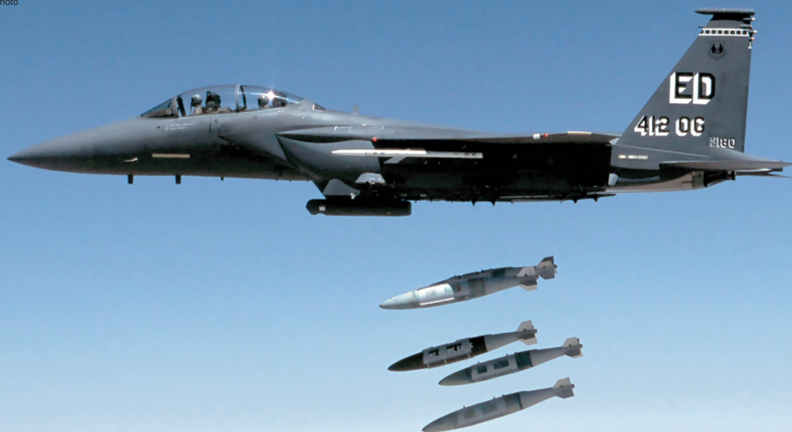
An F-15E drops four JDAMs during a developmental test at Edwards AFB, Calif., in 2002. Precision weapons have become ubiquitous for their accuracy and efficiency.
