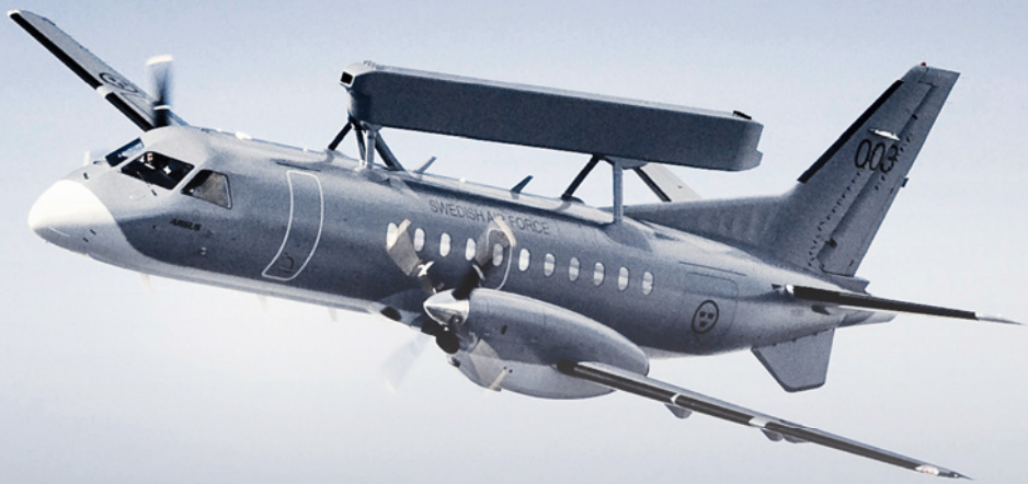
Sweden's Saab 340 Erieye airborne early warning and control aircraft, outfitted with an active electronically scanned array radar system, will need replacing soon.
