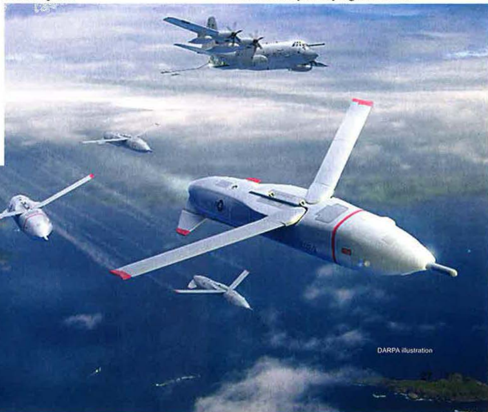
DARPA awarded contracts for the Grem-lins program, which would enable an aircraft to launch several low-cost, reusable unmanned aerial systems with a variety of payloads.
