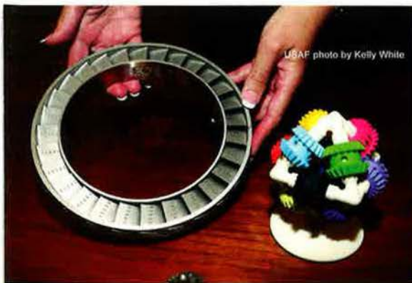
Left: Additive manufacturing with a laser created the titanium part at left, while a 3-D printer made the colorful "Brain Gear" in one piece. Right: A typical 3-D printing setup, including a 3-D printer, a computer, and some examples of 3-D printed objects.
