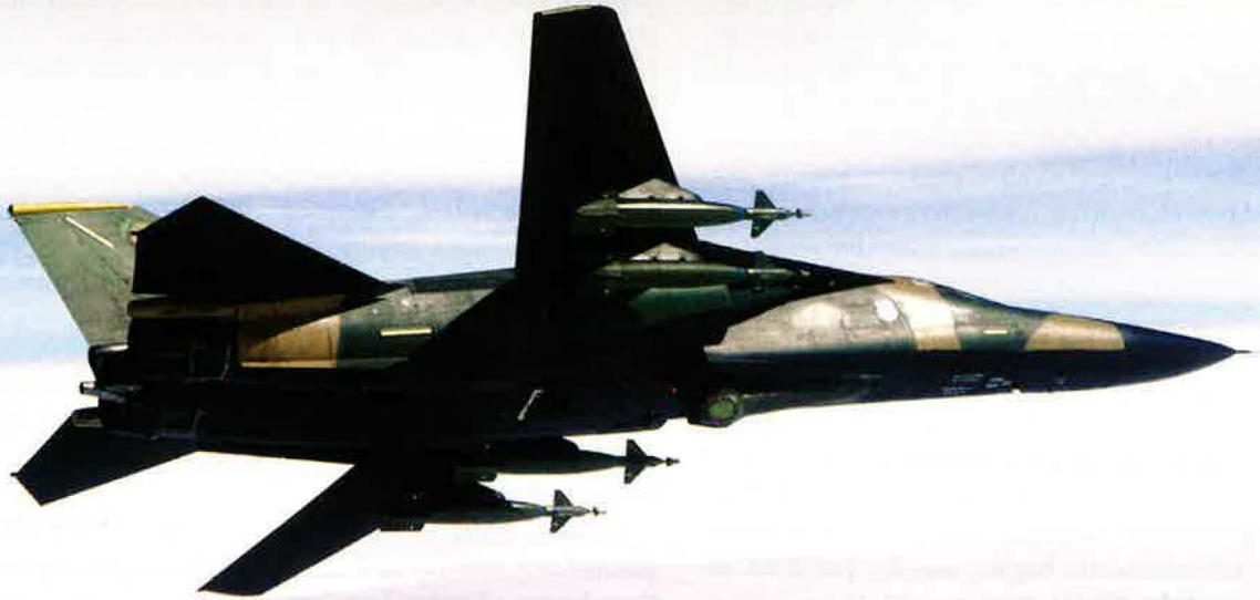
An F-111 carrying four GBU-10 Paveway II bombs and a Pave Tack laser target designator banks over Loch Ness, UK.
