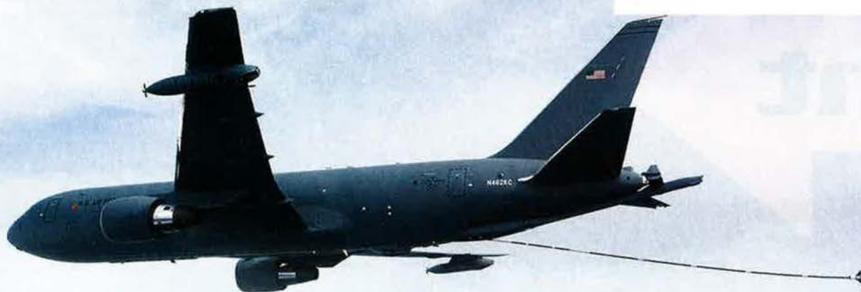
The centerline drogue system and WARP pods will allow the KC-46A to refuel Navy, Marine Corps, and allied aircraft that use the probe-and-drogue system.
