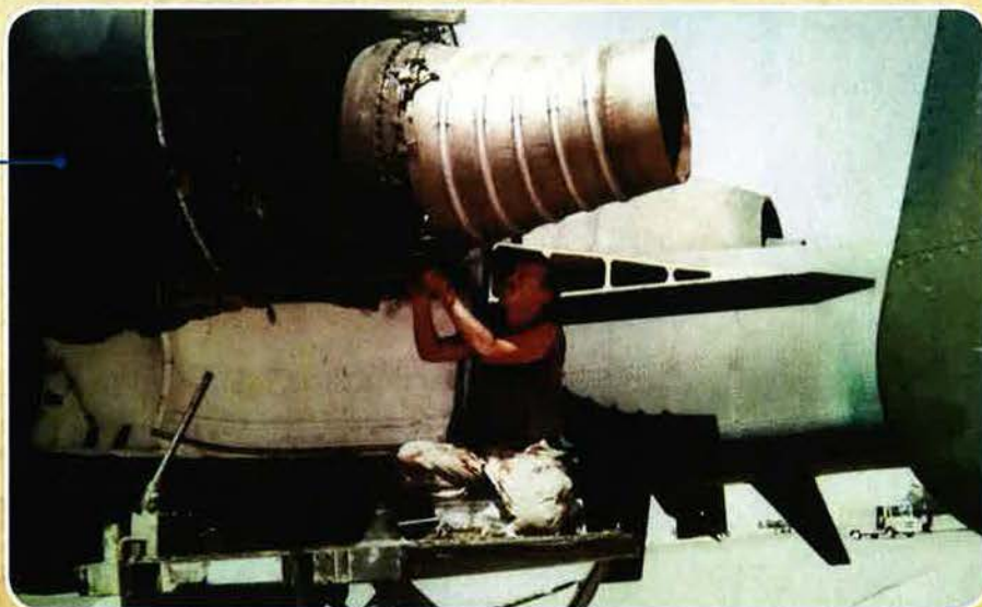
At King Fahd, SSgt. Frederick Schlenker of the 355th Aircraft Maintenance Unit removes a strut while rebuilding the C-sump section of the No. 1 engine in an A-10 from the 354th Tactical Fighter Wing. He was deployed from Myrtle Beach AFB, S.C. Retired SMSgt. Schlenker belongs to the Central Florida Chapter.
