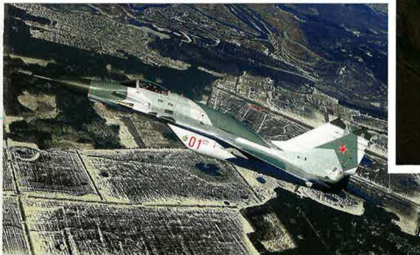
Above: The MiG-29SMT based at Lipetsk is an upgraded version of the early fighter, with new radar, avionics, inflight refueling, and increased fuel capacity (evidenced by the enlarged spine).
