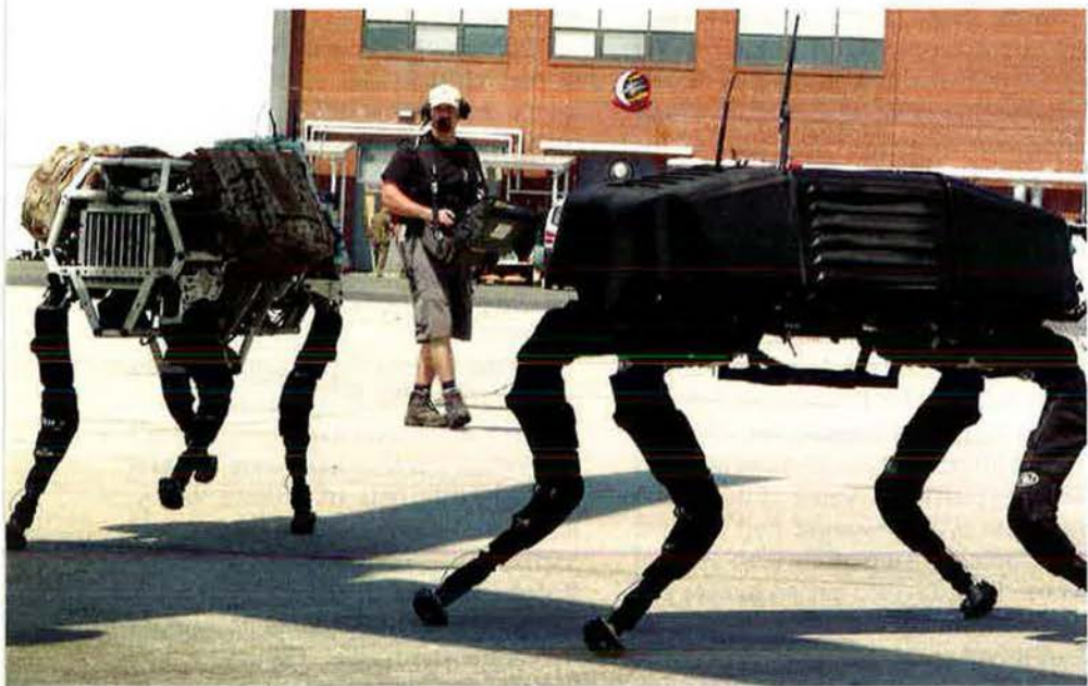
Top: An artist's illustration of Titan Aerospace's long-endurance unmanned airplane called Solara. Google bought the start-up company in 2014. Here: BigDog robots trot around in the shadow of an MV-22 Osprey. The dynamically stable quadruped robots were created in 2005 by Boston Dynamics—a company known for its military robots—and partners. Google acquired Boston Dynamics in 2013.
