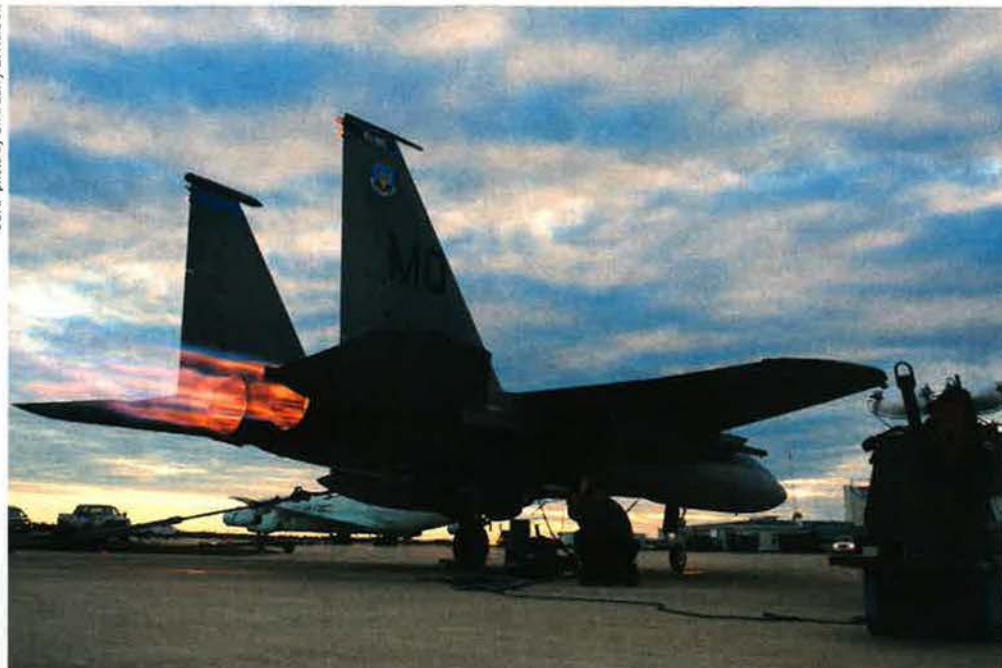
A maintainer conducts an afterburner test on an F-15E during Exercise Maple Leaf in Canada. The median flight hours for the younger F-15E fleet is 9,000.
