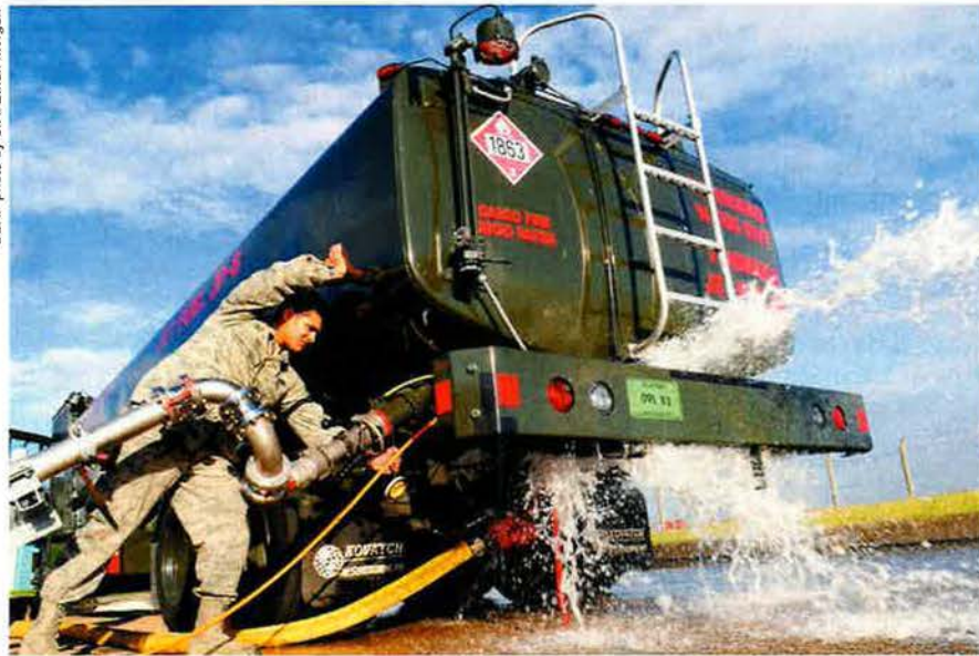
Thar She Blows: SrA. Andrew Leal, a fuels technician with the 100th Logistics Readiness Squadron, shuts off a valve on a fuel truck as liquid spews into the air during a major accident response exercise at RAF Mildenhall, UK. The MARE simulated an accident due to a cracked flange connection during a fuel transfer.
