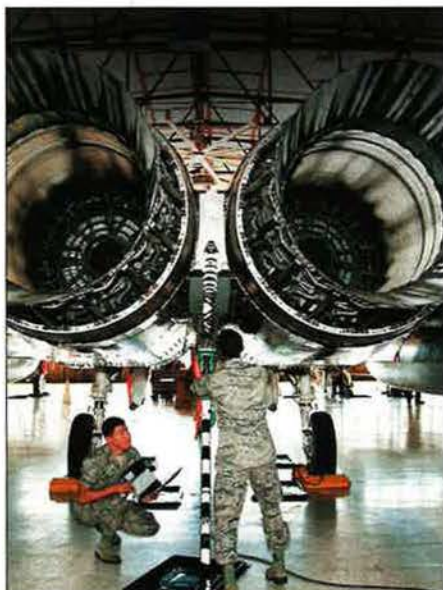
About the cover: Airmen work on a tail-hook damper on an F-15. See "CAF Redo," p. 26. USAF photo by Frank Carter.
