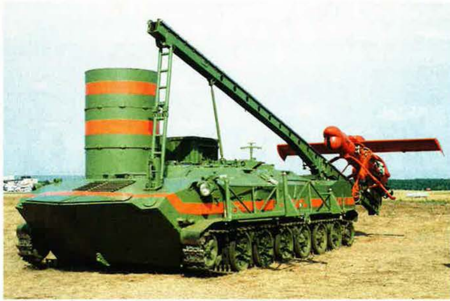
One of Russia's entries into the RPA sector, Yakovlev Pchela, on its launcher. A short-range tactical aircraft, its primary use is battlefield surveillance.
