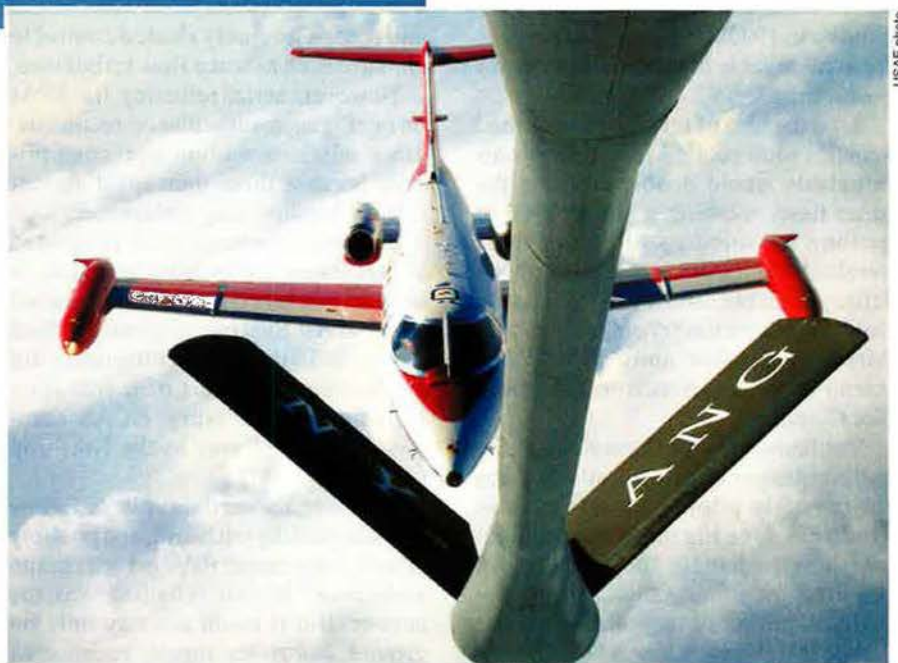
A Calspan Learjet, configured to fly like an RPA, maneuvers into refueling position under a KC-135R in these photos of automated aerial refueling demonstration test flights. By 2007, the system was considered fully successful.
