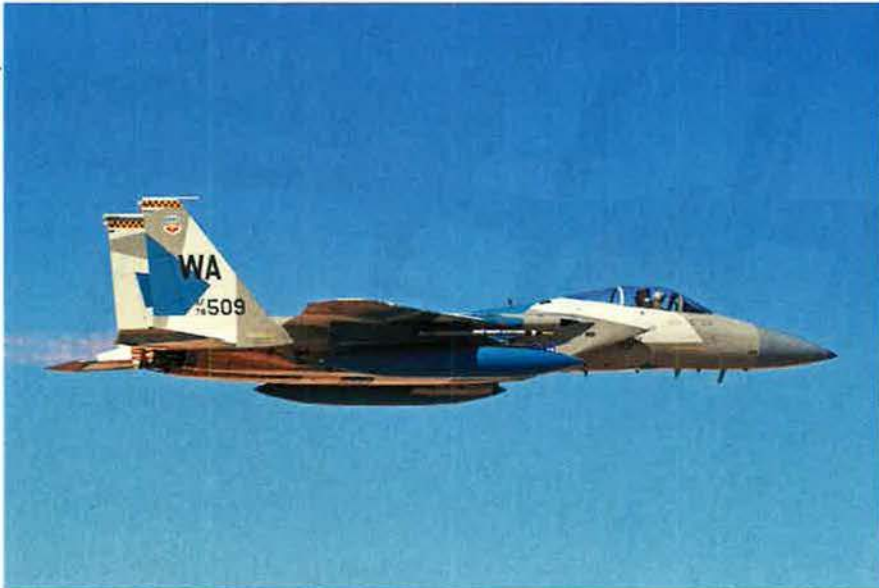
Wait, Who's That?: An F-15C, wearing one of the new "Splinter" paint schemes, heads out on a Red Flag mission at Nellis AFB, Nev. The design mimics Russian fighters such as the Su-35 and T-50 PAK FA and is meant to provide an even more realistic threat to the Blue Forces during the training exercise.
