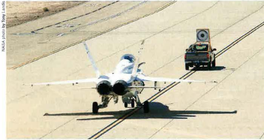
The F/A-18 research aircraft follows a pickup carrying an airborne tanker drogue image down a runway in early AARD testing. An RPA's approach to the boom is broadly based on optical recognition, aided by algorithms to improve prediction accuracy.
