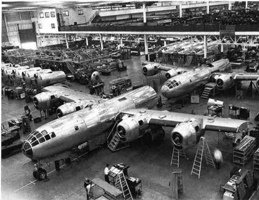
B-29 wings are mounted in the factory. The Superfortress was a complex, sophisticated aircraft that required a huge, well-trained workforce.
