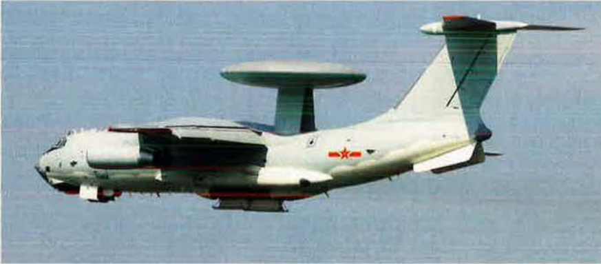
In 2006-07, China commissioned four KongJing-2000 aircraft. The AWACS aircraft are based on the airframe of the Russian-made A-50/II-76MD.
