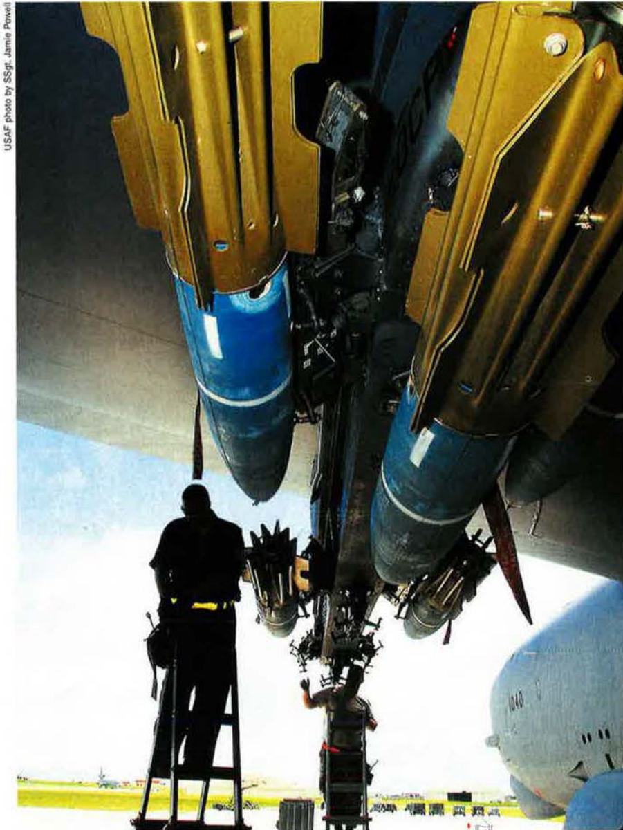
SSgt. Dustin Hyden (l) and SSgt. Doyle Atkinson load Mk 62 naval mines onto a B-52 in preparation for a joint exercise with the Navy. The nuclear-capable aircraft is remarkably versatile.
