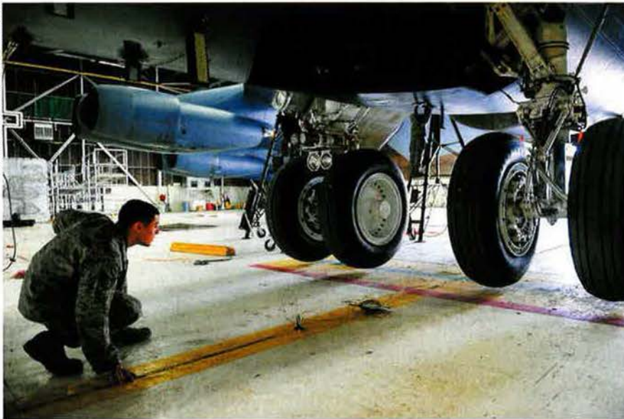
SSgt. Jon Alместica watches a B-52 being carefully lifted off the ground at Minot. The aircraft's struts and seals were replaced during routine maintenance.
