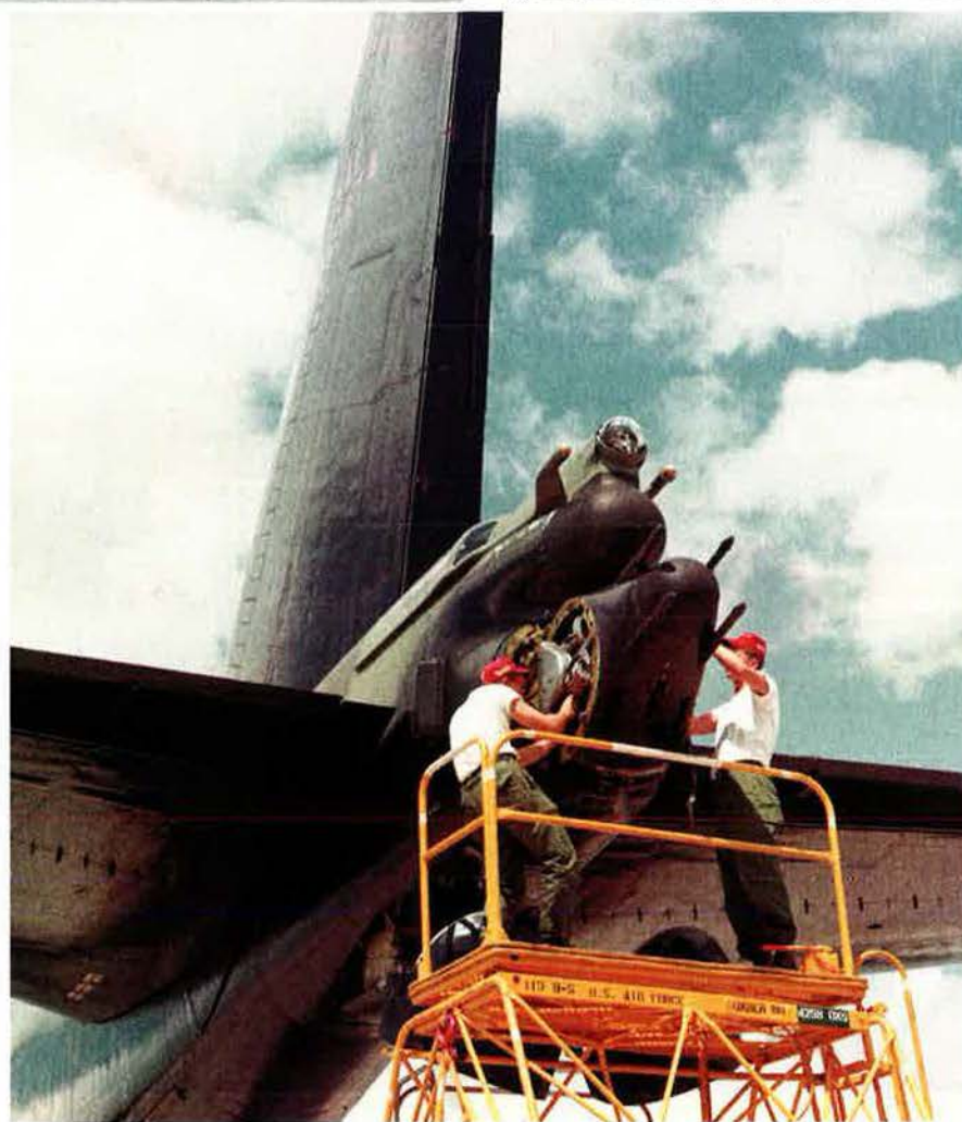
Above: A B-52F rolls out (back). In the foreground is a tail detail, showing, from left to right, the ammunition access door, the drag chute compartment, and the gunner's entry hatch. Right: Maintainers service the four .50-caliber M3 machine guns in the tail of a BUFF.
