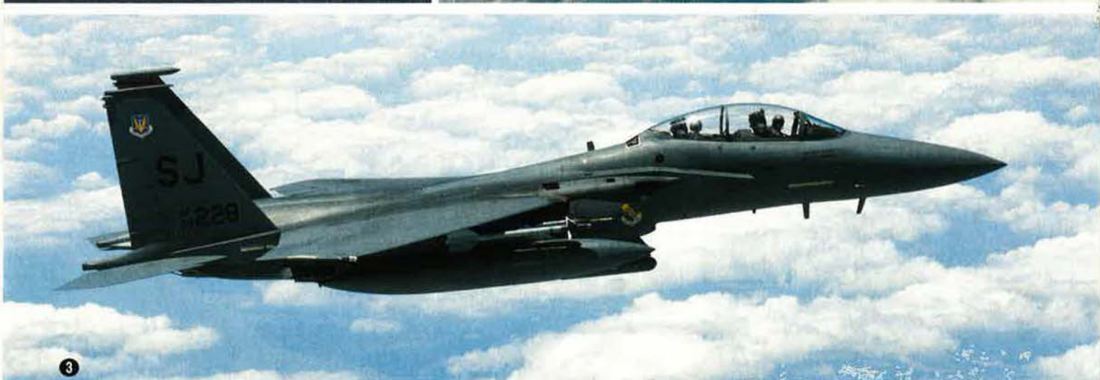
1 An F-15E gets airborne. More than 63 feet long and with a max takeoff weight of 81,000 pounds, the F-15E is huge for a fighter. The upper fuselage between the vertical tails is sometimes referred to as "the tennis court." 2 A 916th tanker maneuvers with an F-15E for
