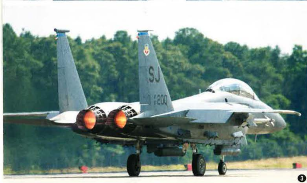
11 A landing F-15E deploys its huge dorsal airbrake, known as the "board," to slow its speed and rollout. The pilot will also hold the nose up to slow the big jet aircraft down. 12 A1C Kelsey Brown disconnects a grounding wire on an F-15E. 13 Afterburners lit, an F-15E prepares to blast off on a training flight, carrying LANTIRN pods and a Sidewinder air-to-air missile. 14 A 333rd Strike Eagle pulls up to a tanker.
