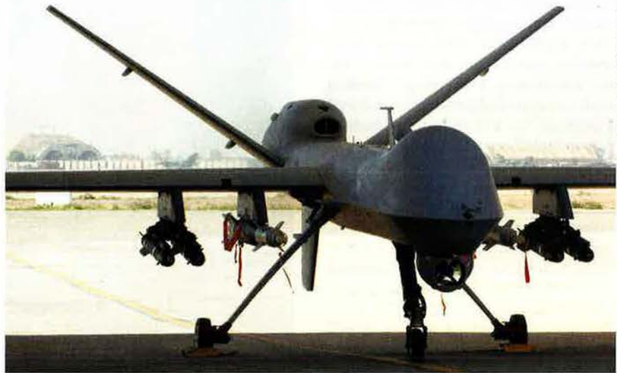
Top: An E-8 JSTARS aircraft over Robins AFB, Ga. JSTARS uses a multimode side-looking radar to detect, track, and classify moving targets behind enemy lines. Above: An MQ-9 Reaper in a shelter at JB Balad, Iraq. Intelligence-surveillance-reconnaissance capabilities such as those offered by these aircraft are expensive and always in high demand.
