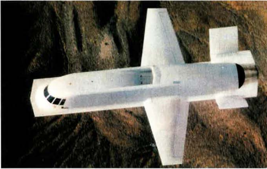
Tacit Blue, Northrop Grumman's stealthy battlefield control technology demonstrator aircraft on one of its 135 flights, which began in 1982.
