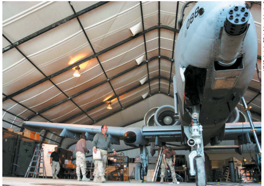
Maintainers with the 104th Expeditionary Fighter Squadron work on an A-10 undergoing contingency phase maintenance at a deployed location. A-10s have provided critical close air support throughout OEF.
