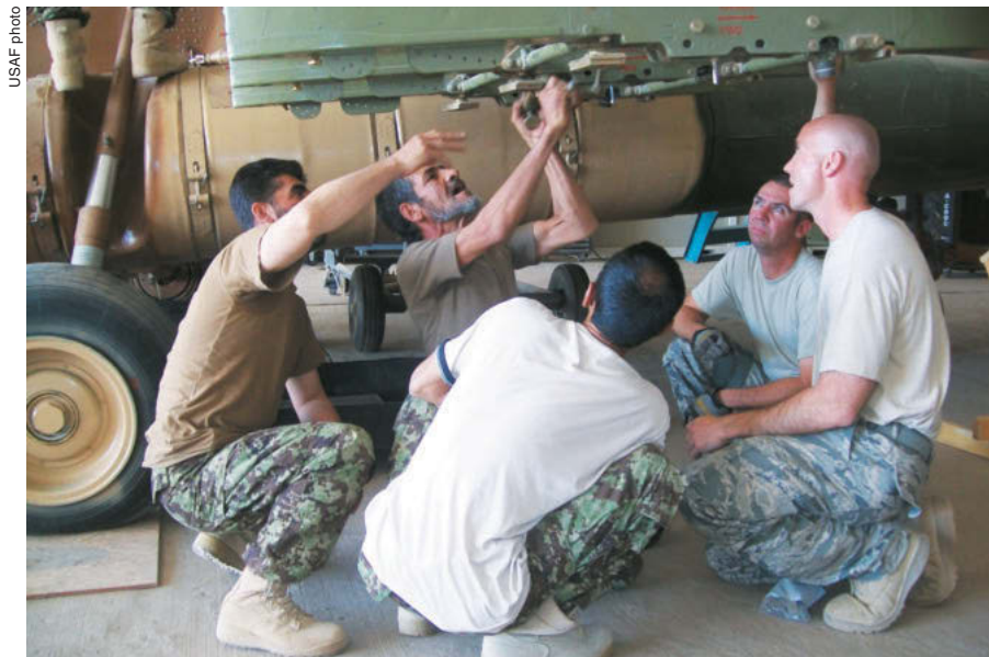
MSgt. Ben Fitzgerald and MSgt. Timothy Brizedine teach members of the Afghan Air Force how to install a sway brace to keep rocket pods from shifting during flight, at Shindand AB, Afghanistan. US airmen are serving as instructors and mentors to Afghan airmen as part of a NATO training mission to teach the Afghan maintainers how to prepare and install Mi-17 weapons pylons and rocket pods.
