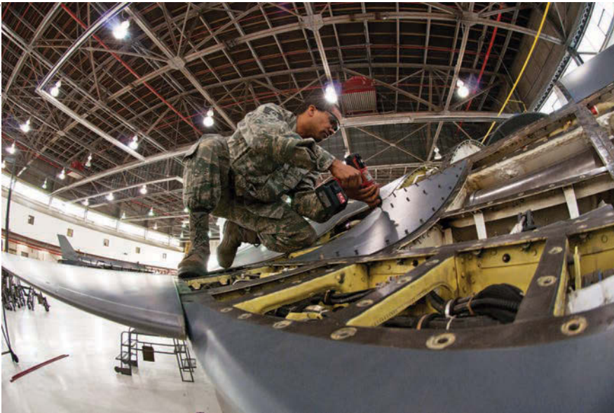
SSgt. Ebon Mitchell attaches body panels to an F-16 during a 300-hour phase inspection at JB Andrews, Md. The ANG's F-16 Block 30s had been slated to retire by 2018.
