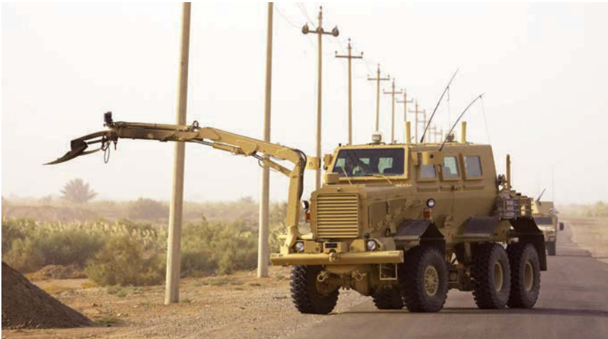
The arm on a Buffalo mine-protected vehicle reaches for a suspected IED. Buffalos can make it safer to unearth an IED but cannot replace a trained EOD technician's ability to distinguish hazards on foot.
