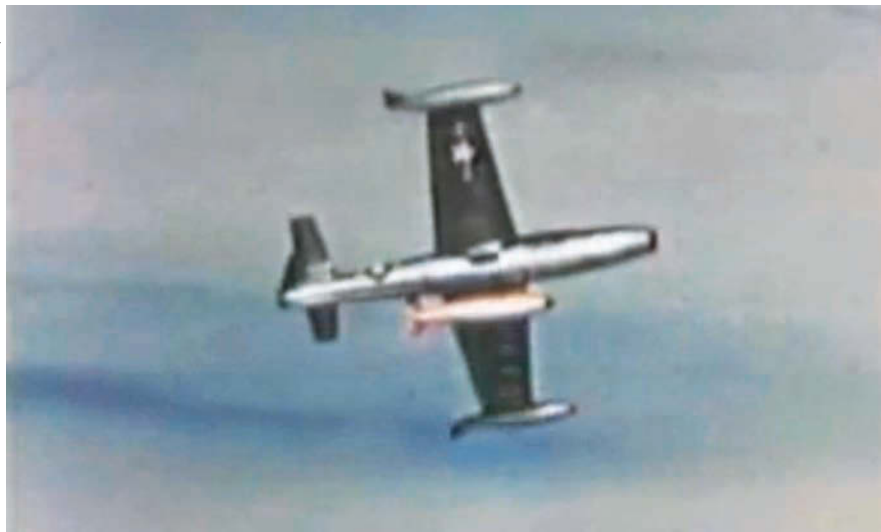
An F-84 carries a 30-inch nuclear weapon. The newly miniaturized nukes weighed just 1,680 pounds, far lighter than the weapons designed to be carried on bombers.
