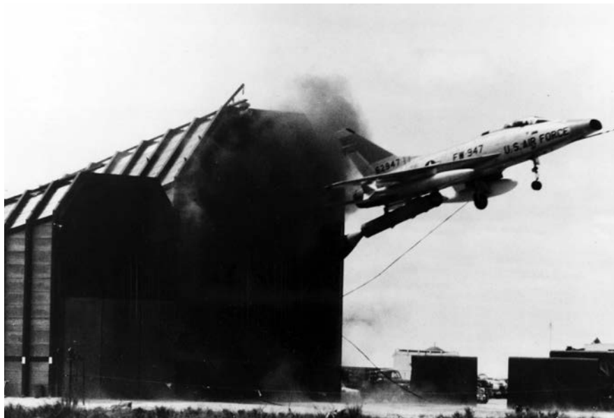
A zero-length launch of an F-100D. Note the "special weapon shape" under the left wing. The F-100 took on the nuclear mission from the F-84.
