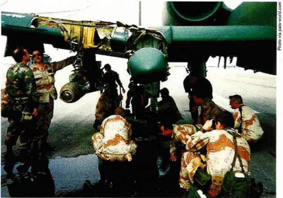
Airmen examine Johnson's A-10, mangled on a later mission over Iraq. He managed to refuel in flight and wrestle his Hog back to base in Saudi Arabia.
