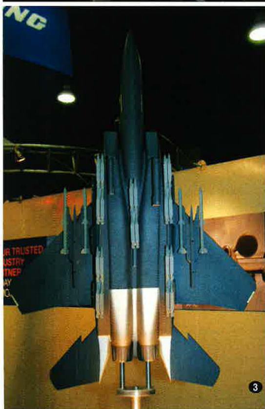
11 Honeywell's F124 turbofan engine powers light combat and trainer aircraft. 12 At AFRL's exhibit (left to right) A1C Thaddeus Majtyka, A1C Drake Solomon, and SrA. Maria Carlson, all crew chiefs, get briefed on the Small Diameter Bomb. 13 Boeing's F-15E shows off its ability to carry 20 Small Diameter Bombs, plus sensors and air-to-air missiles. Many models evidenced the trend toward smaller, more accurate weapons. 14 A trio of F-35 models, representing the Air Force, Navy, and Marine Corps versions, show off their ability to carry external stores and internal weapons payloads. 15 Maj. Amy Nesbitt (r), from Air Force Headquarters at the Pentagon,
