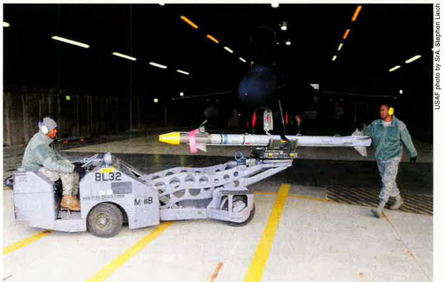
Load 'er Up: SrA. Marquell Stalling drives an MJ-1 weapons loading vehicle as SSgt. Eric Venter guides an AIM-9X missile in an aircraft hangar at Keflavik, Iceland. The airmen were part of a NATO allied forces air policing mission to Iceland.
