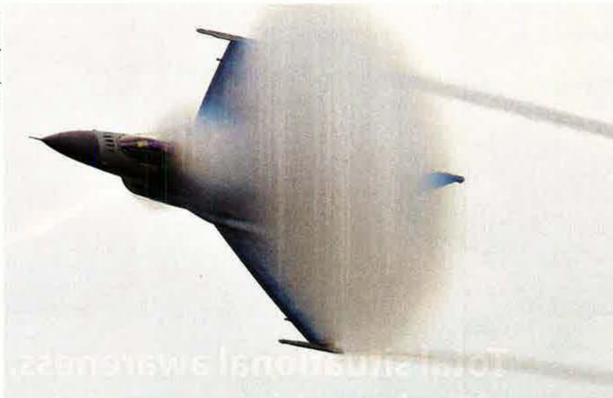
Vaporized: An F-16 creates a "cone" of condensation as it nears Mach 1 during a flyby at an open house at the Air National Guard's Volk Field ANGB, Wis. The cone appears as jet aircraft experience a sudden drop in pressure at high speed.
