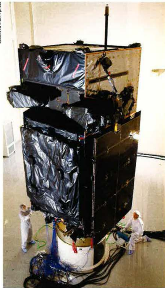
SBIRS GEO-1 is prepared for thermal vacuum testing at a Lockheed Martin Space Systems facility.
