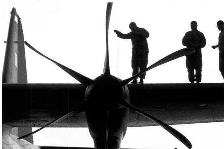
Tip to Tail: Maintainers perform an isochronal inspection on a C-130J Super Hercules at Ramstein AB, Germany. The inspections are in-depth looks at—and into—every aspect of the aircraft. They last 10 days, are performed every 420 days, and take about 60 airmen from many career fields to perform.
