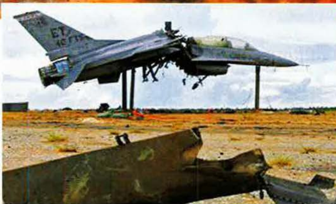
Boom Goes the Dynamite: An F-16 bursts apart in an explosion on the range at Eglin AFB, Fla. The controlled blast was a static test of the flight termination system to be installed on the future QF-16, a supersonic, reusable, full-scale aerial target drone to be modified from an F-16. Under evaluation was the system's ability to immediately and fully terminate a flight. The test also helped determine a "debris footprint" for safety purposes.
