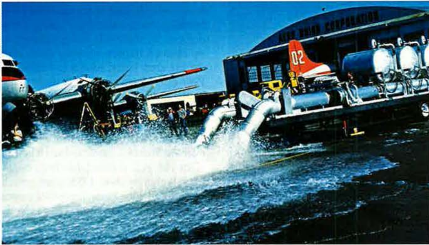
The Modular Airborne Firefighting System dumps hundreds of gallons of water on the ramp during a test at Chico, Calif., in 1985.
