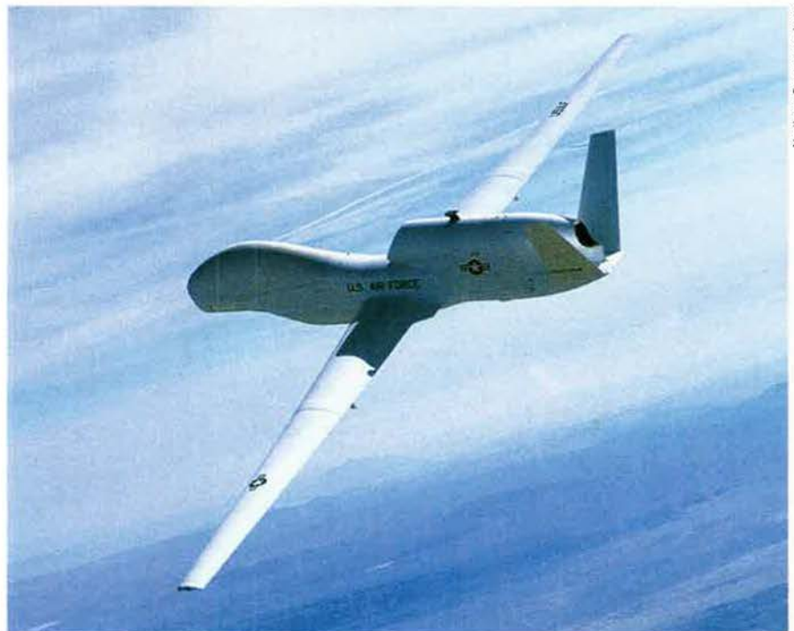
The RQ-4 Global Hawk (here, in test flight) started out as an experiment but has been improved steadily using the block upgrade approach.
