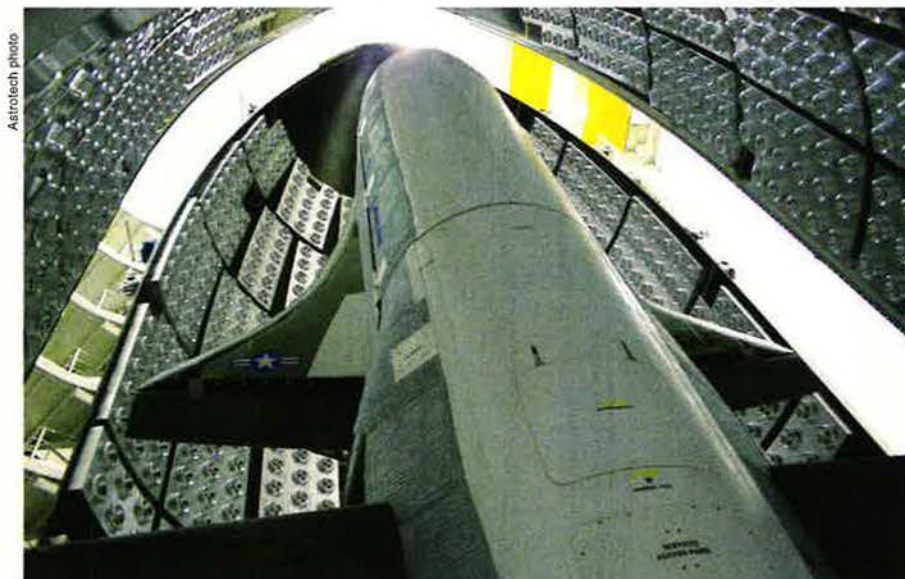
The X-37B Orbital Test Vehicle, shown at the Astrotech Corp. facility in Titusville, Fla. Officials hope this unmanned space vehicle will provide orbital reusable access, not unlike a fighter for space flight.
