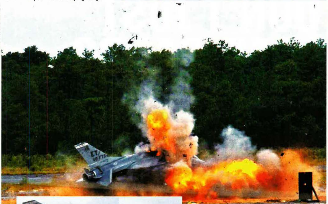
Boom Goes the Dynamite: An F-16 bursts apart in an explosion on the range at Eglin AFB, Fla. The controlled blast was a static test of the flight termination system to be installed on the future QF-16, a supersonic, reusable, full-scale aerial target drone to be modified from an F-16. Under evaluation was the system's ability to immediately and fully terminate a flight. The test also helped determine a "debris footprint" for safety purposes.
