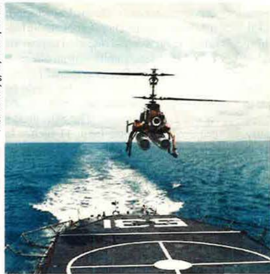
A remotely operated DASH comes in for a landing on the deck of a US Navy destroyer. Plans called for DASH to deliver a nuclear depth charge.
