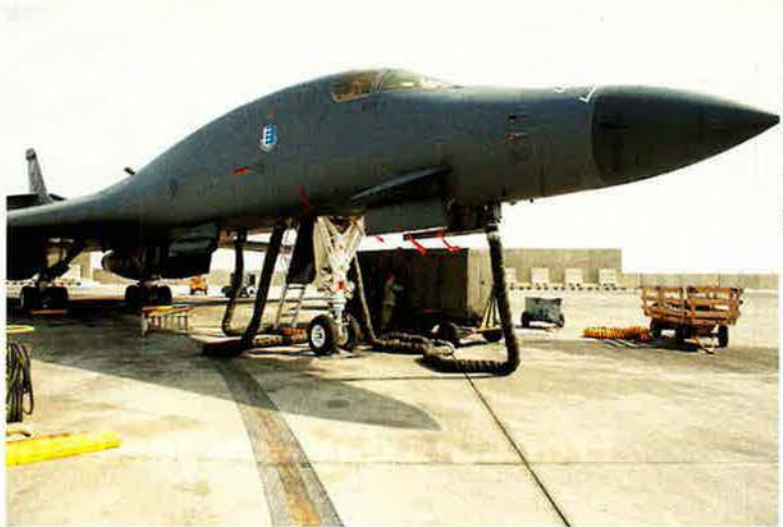
Left: SSgt. Richard Mabry carefully inspects a B-1 wheel bolt for cracks. Above: TSgt. Jesse Maddox installs an air-conditioning "splitter" on a B-1. The device allows the aircraft to only use one air-conditioning unit instead of several.
