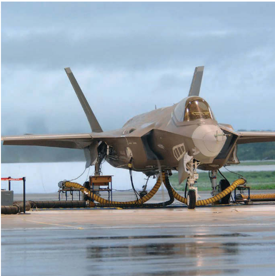
An F-35 undergoes an engine test run.
