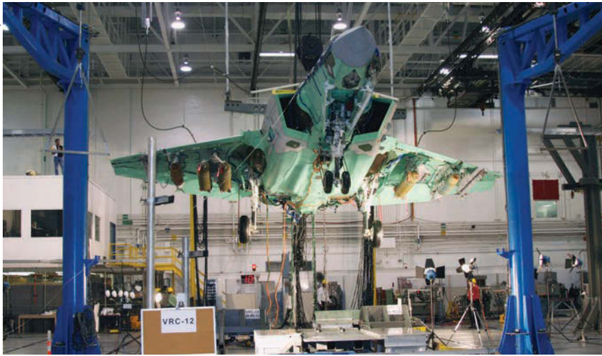
The Navy's F-35 variant is put through structural integrity testing during a drop test at Lockheed's test facility.
