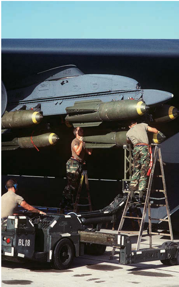
Airmen load a Mk 117 bomb onto a B-52 Stratofortress during prewar preparation.
