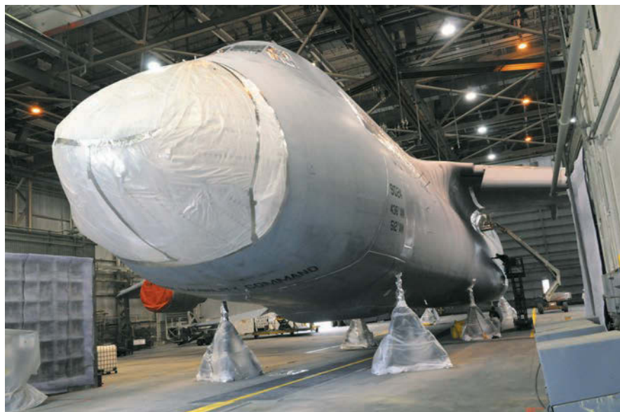
A Galaxy is masked in preparation for paint removal. Sharply improved C-5 reliability will give USAF the equivalent of dozens more airlifters.
