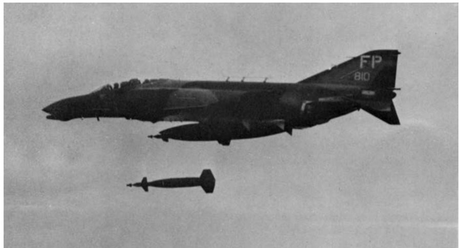
An F-4 drops a Mk 84 laser-guided bomb. F-4s such as this one loaded with precision weapons took down the Dragon’s Jaw bridge.
