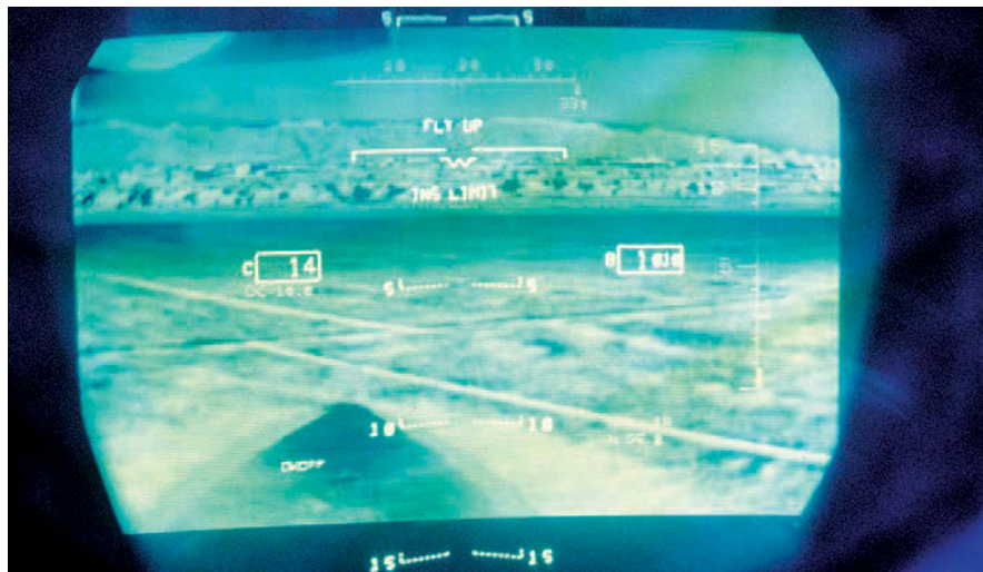
Infrared image of a nighttime target, seen on an F-15E head-up display. Use of such systems to deny enemies respite from attack, combined with innovative tactics, have helped USAF keep down its own attrition and raise mission success rates.
