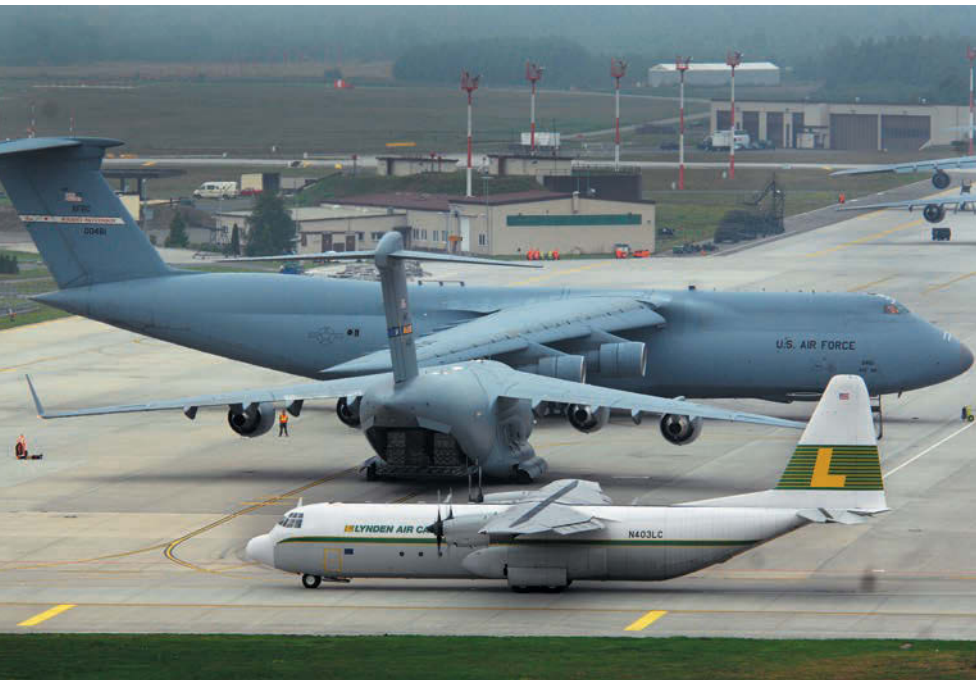
Shown, back to front, are a C-5, C-17, and “stretched” C-130. Modified with a major upgrade, C-5Ms like the one below broke time-to-climb records and moved massive amounts of cargo in a surge exercise.
