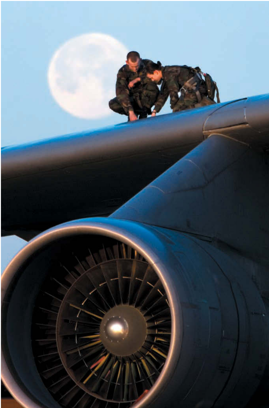
A1C Justin Fleming (l) and Amn. Alisha McKinney change a fuel probe on a C-5's wing. Galaxys receiving new engines will require fewer maintainers.
