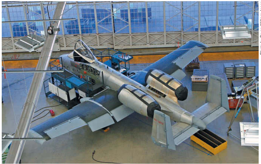
A multibillion dollar program is under way to replace the worn-out wings on 1980s-era A-10s such as this one. A dove-tailing digital upgrade gives the aircraft capability for new sensors and weapons.
