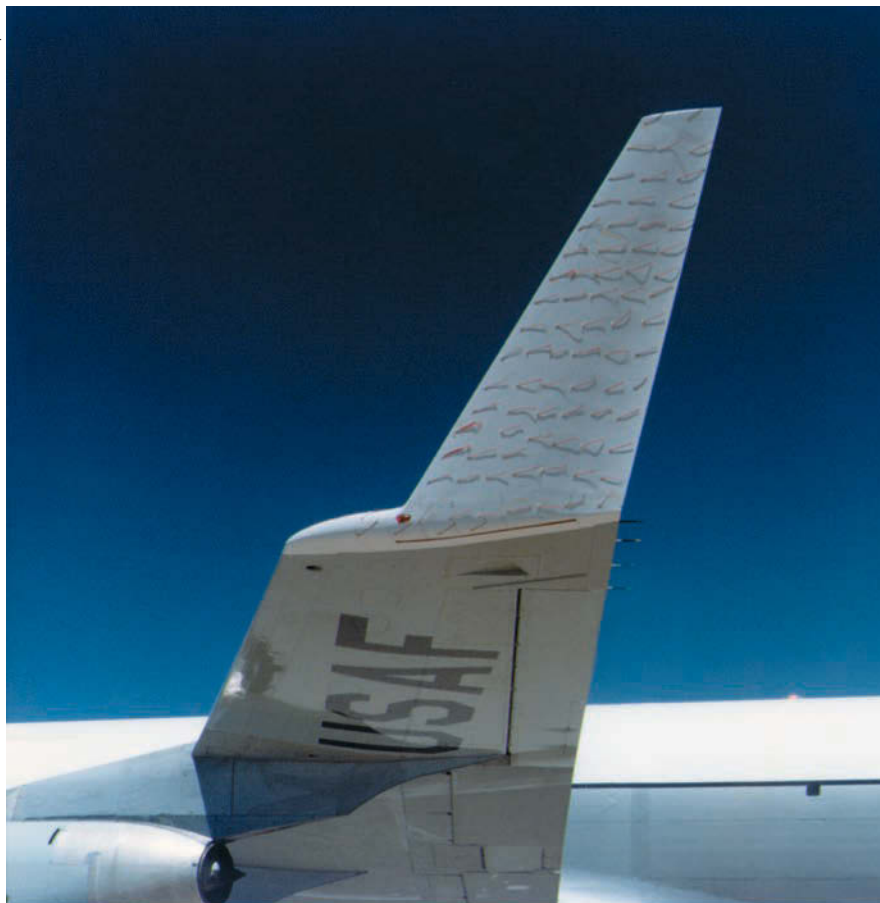
The winglet (seen here in testing on a KC-135) later became crucial to the C-17's performance. Seemingly simple, the winglet adds lift far beyond its cost in weight, and has been adopted on many airliners.
