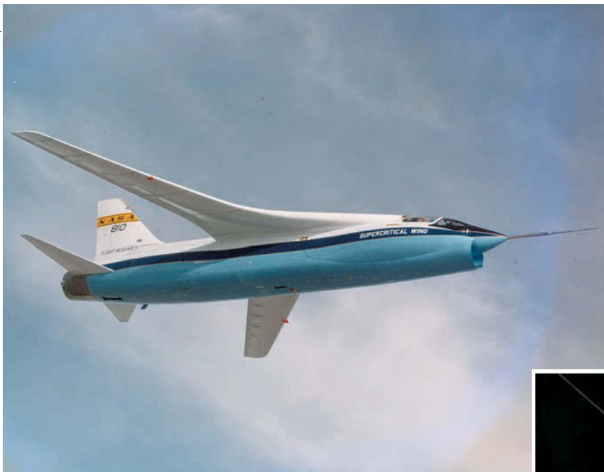
Whitcomb with a wind tunnel model of a TF-8 configured with his supercritical wing (below), and NASA's flying version (left). His innovation has saved billions of dollars in fuel costs.
