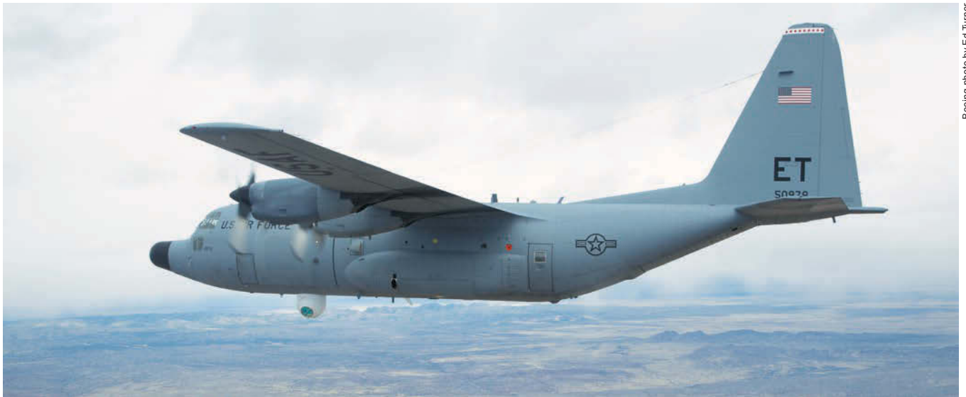
A C-130 carrying the Advanced Tactical Laser prepares for a test near Albuquerque, N.M.
