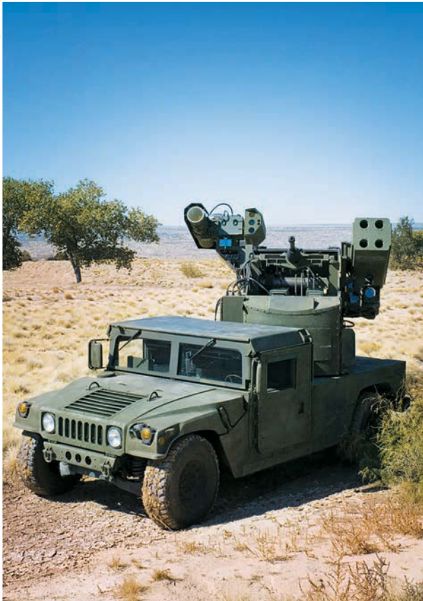
Above and right: Boeing's Laser Avenger system integrates a directed energy weapon with an Avenger air defense system. Laser Avenger can detonate unexploded ordnance or an improvised explosive device while troops stay inside the vehicle.
