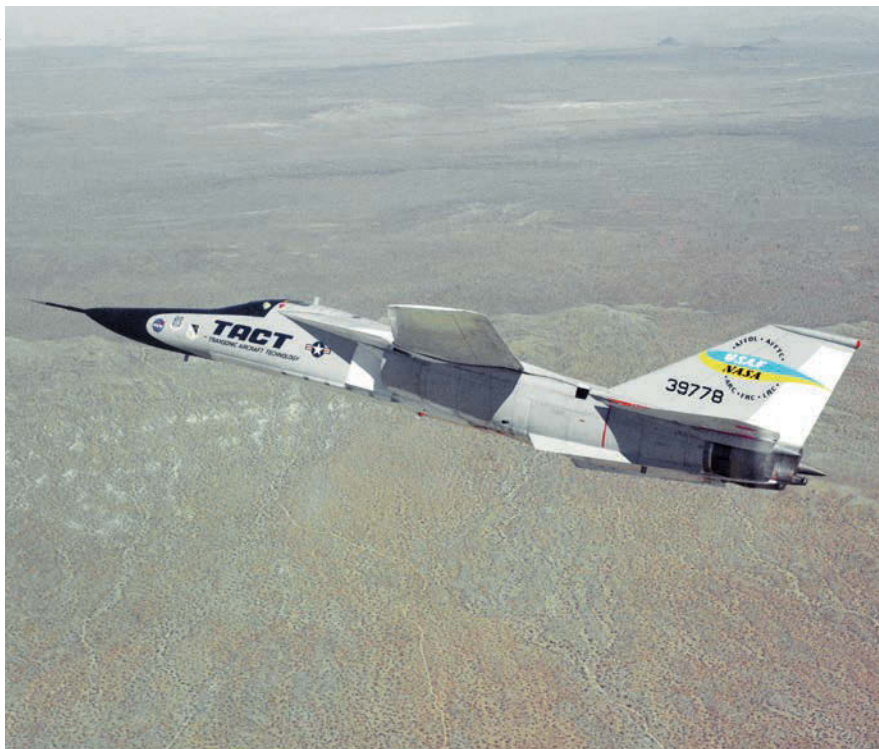
A swing-wing Transonic Aircraft Technology (TACT) F-111A configured with Whitcomb's supercritical wing. It delivered 50 percent better lift than the standard F-111A.
