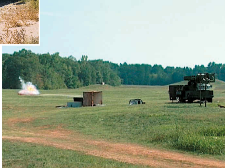
Above and right: Boeing's Laser Avenger system integrates a directed energy weapon with an Avenger air defense system. Laser Avenger can detonate unexploded ordnance or an improvised explosive device while troops stay inside the vehicle.
