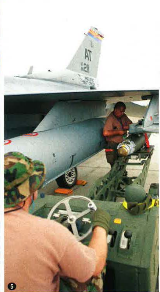
F-15s and helicopters to bombers. The Litening targeting pod and the Situational Awareness Data Link are just two systems first explored by the AATC that have now spread into the active force. 15| MSgt. Ruben Perez secures a JDAM to a BRU-57 rack for a test mission as TSgt. Harold Lewis maneuvers the loader.
