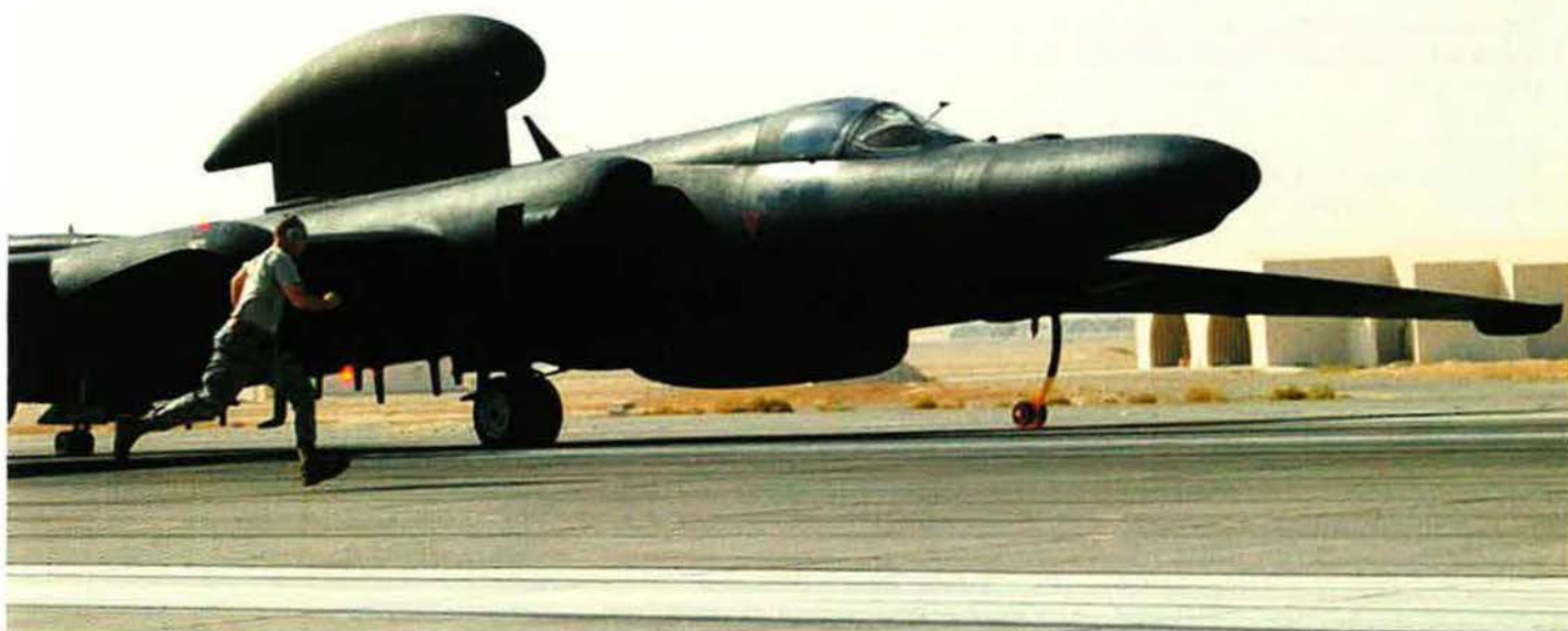
At an unidentified Persian Gulf air base, two USAF airmen prep a U-2S spyplane for imminent takeoff. The aircraft and pilot, Capt. Peter Gryn, were deployed from Beale AFB, Calif., to the 380th Air Expeditionary Wing. U-2s, with a wingspan of 103 feet, can fly above 70,000 feet to provide intelligence-surveillance-reconnaissance data for combatant commanders and individual troops alike. This particular U-2, No. 68-10337, exceeded 25,000 flying hours on a mission flown two weeks after this photo was snapped.
