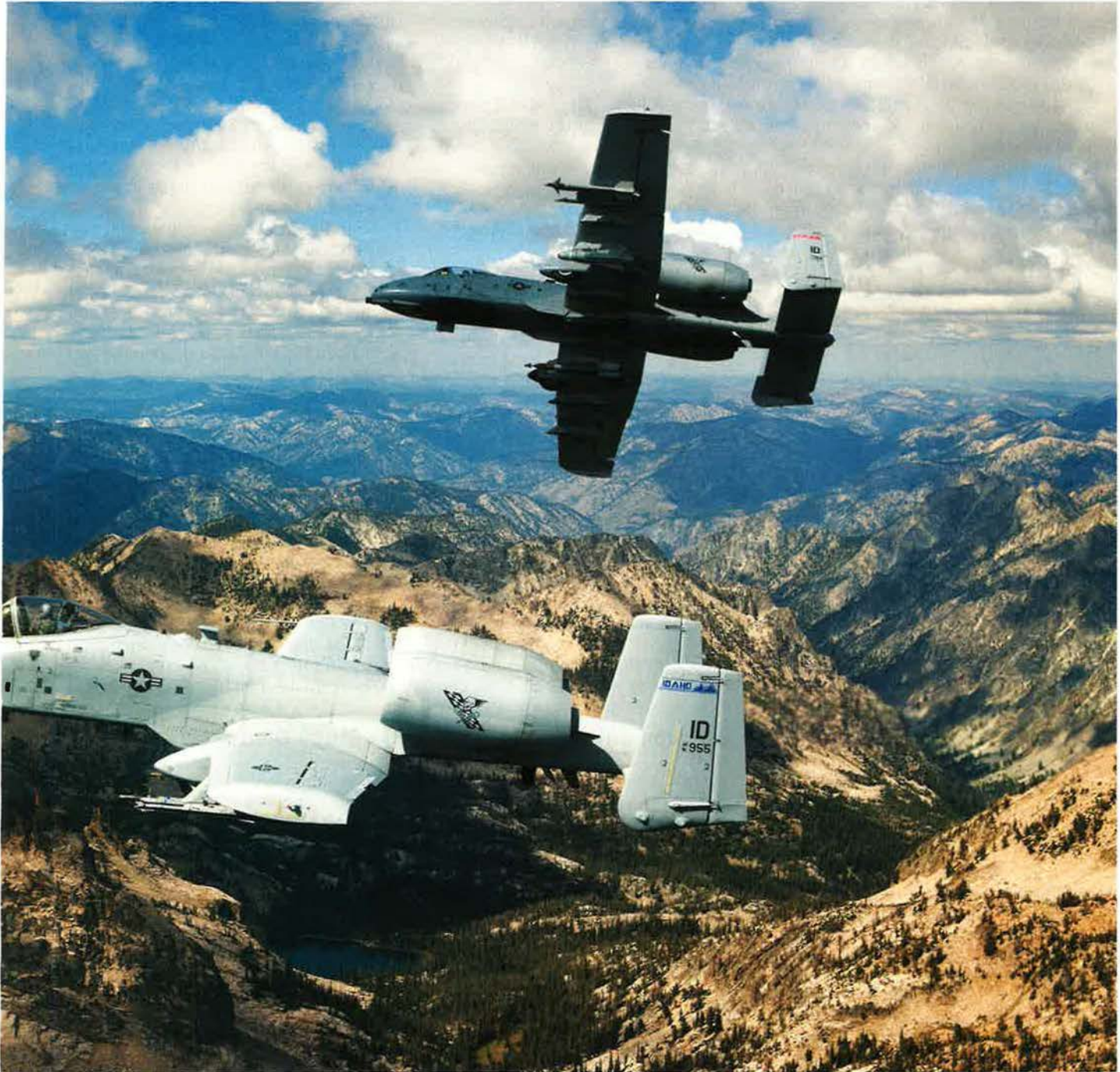
Two newly minted C models of the A-10 attack aircraft—both assigned to the Idaho Air National Guard’s 124th Wing in Boise—maneuver over the rugged Sawtooth Mountains. For a year, the wing’s 190th Fighter Squadron has been upgrading from A-10A Warhogs to the A-10C model. The C has new “glass cockpit” displays, radio equipment, data link, and precision engagement mods. The latter allow pilots to identify and strike targets from higher altitudes and greater distances, using highly accurate weapons.
