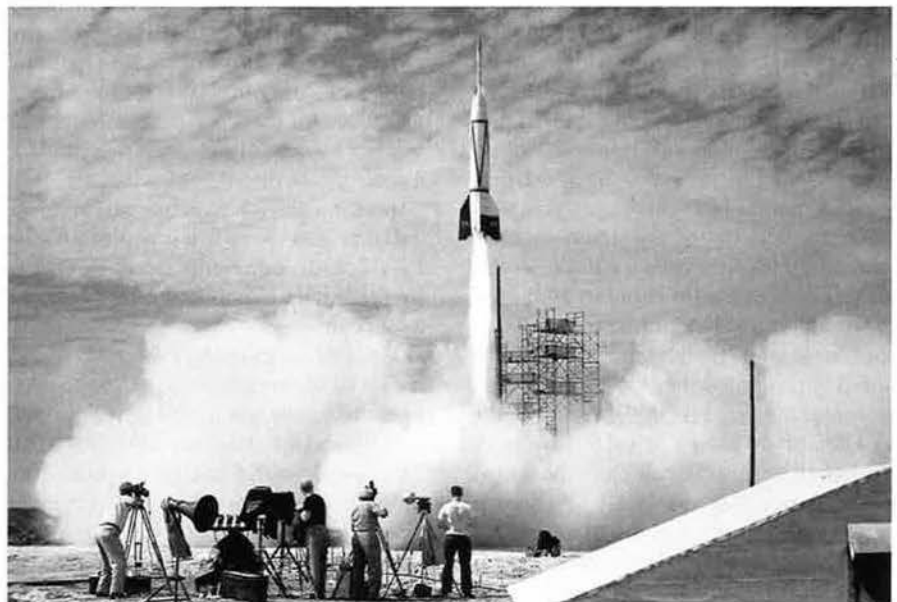
The 1950 launch of the first rocket from Cape Canaveral, Fla., shown here, was a WAC Corporal rocket atop a V-2.
