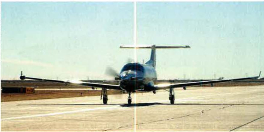
PC-12 Pilatus aircraft, such as the one pictured here, are versatile and have the ability to operate on short and unimproved runway surfaces.
