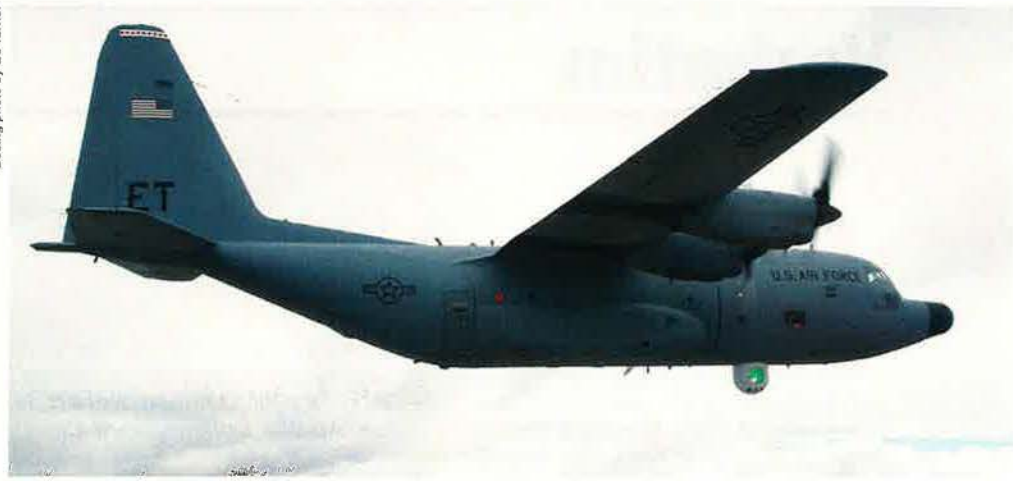
A C-130H modified to carry the Advanced Tactical Laser goes through tests over Albuquerque, N.M.
