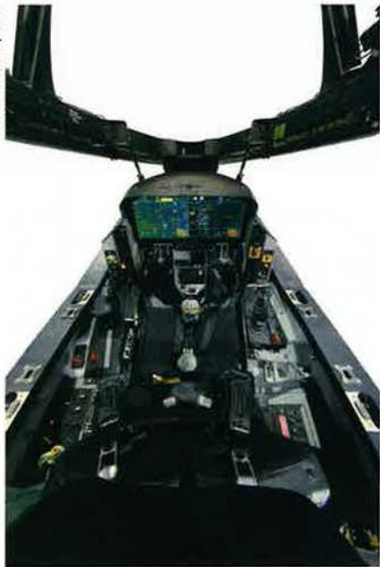
Cockpit displays will complement data projected on the pilot's helmet. Variants will have nearly identical layouts.
