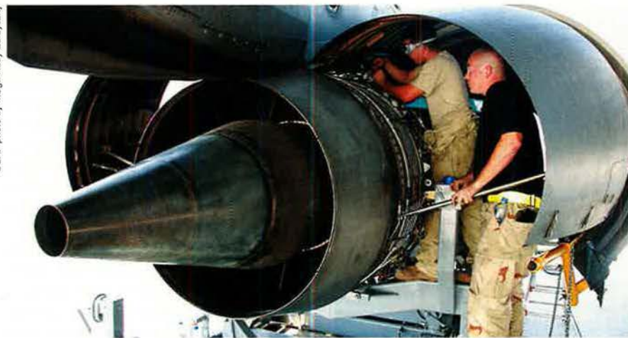
A1C Louis Martens (l) and SSgt. Joseph Dodson (r) install safety wires on the engine mounts of a replacement engine for a KC-10.
