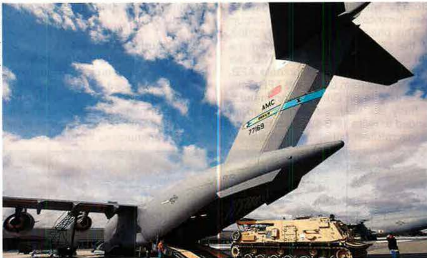
It's Got Versatility: Contractors at Dover AFB, Del., direct an Army M88A2 HERCULES heavy equipment recovery vehicle into a C-17 Globemaster III. The C-17 is the most flexible of USAF's heavy lifters, and can deliver troops and all types of cargo to main operating bases or directly to forward operating locations.
