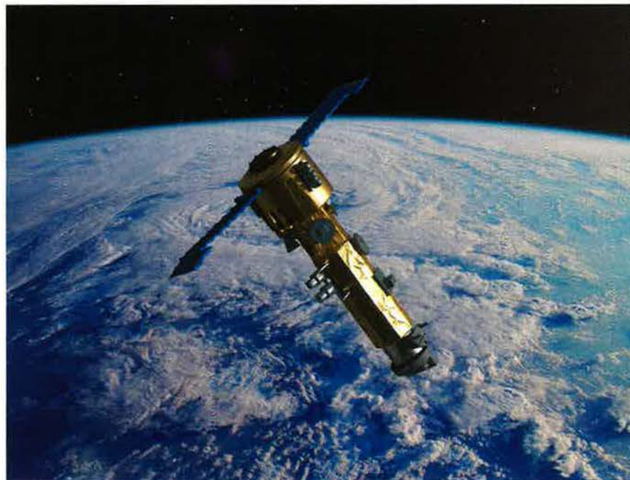
TacSat-2, already in orbit, features a variety of instruments, including a low-power imagery sensor and a signals intelligence payload.
