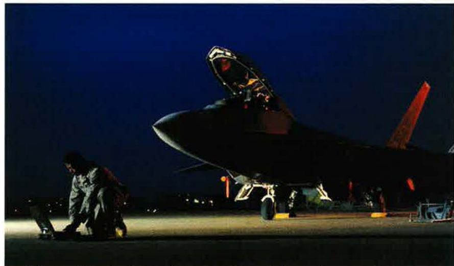
Tapping Diagnostics: A1C Aaron Tate, assigned to the 27th Fighter Squadron based at Langley AFB, Va., uses a portable maintenance aid to run a check on an F-22 Raptor at Kadena AB, Japan. Maintainers can plug the new laptop computer-like devices into aircraft and review oil and fuel levels, diagnose problems, and perform auxiliary power unit ground operations.
