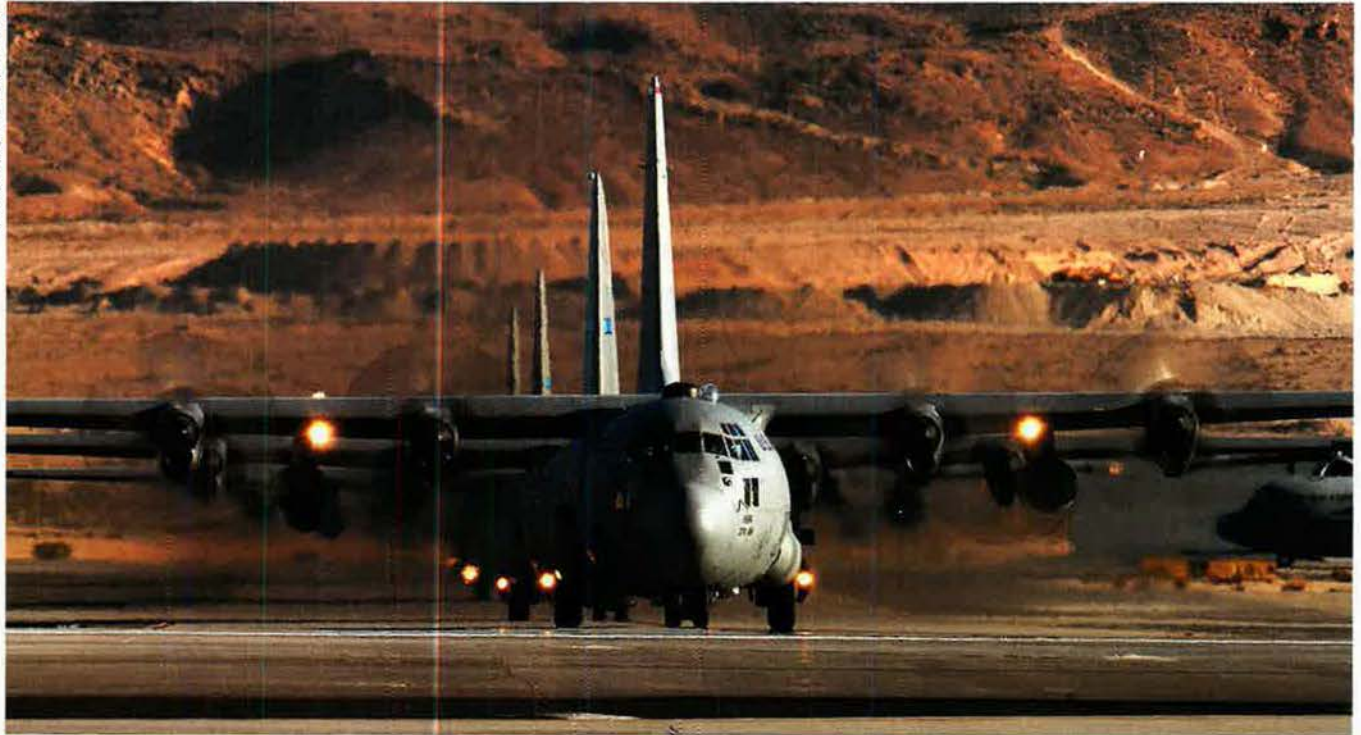
Lining Up To Help: C-130s taxi at Nellis AFB, Nev., after a training mission. C-130s such as these provide intratheater airlift in Afghanistan, Iraq, and the Horn of Africa. The aircraft is capable of operating from rough strips and is the prime transport for air-dropping troops and equipment into hostile areas.
