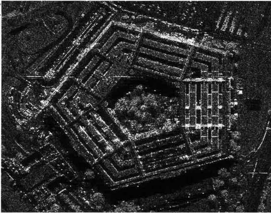
A high resolution airborne synthetic aperture radar image of the Pentagon, Arlington, Va. In the 1970s, earlier airborne radar imagers gathered intelligence on targets in Cuba.
