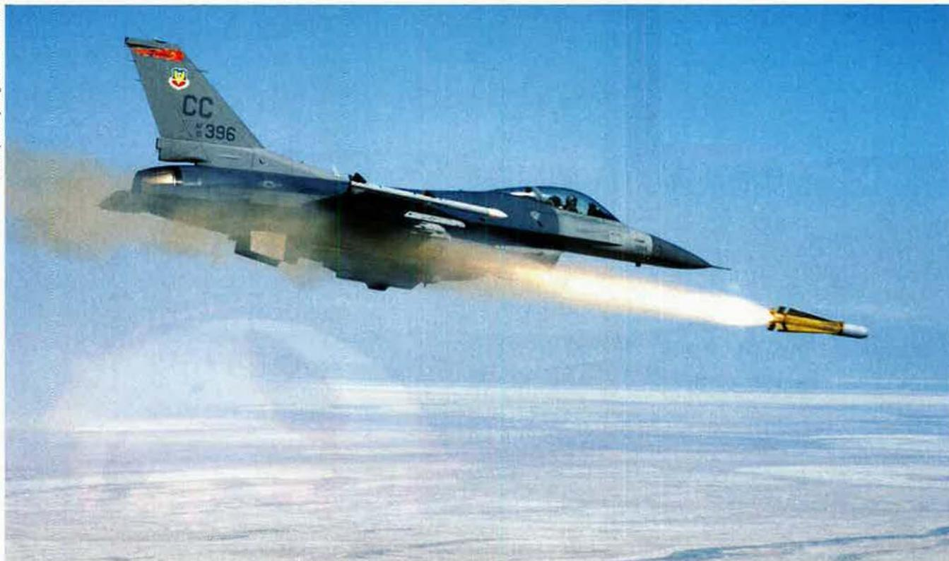
**An F-16 fires an AGM-65H Maverick missile at a target at the Utah Test and Training Range. New Mavericks are being used against moving targets such as terrorists' trucks.**
