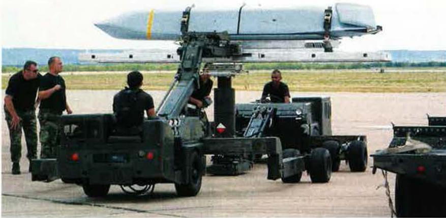
Airmen at Dyess AFB, Tex., ready a Joint Air-to-Surface Standoff Missile (JASSM) to be loaded onto a B-1B.
