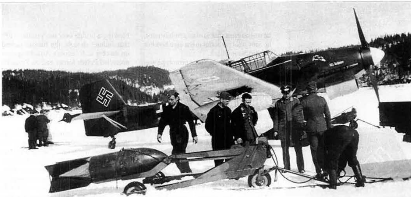
The Ju 87R, pictured here in the Norwegian campaign, was equipped with underwing fuel tanks to extend its range—all the better to terrorize shipping lanes.
