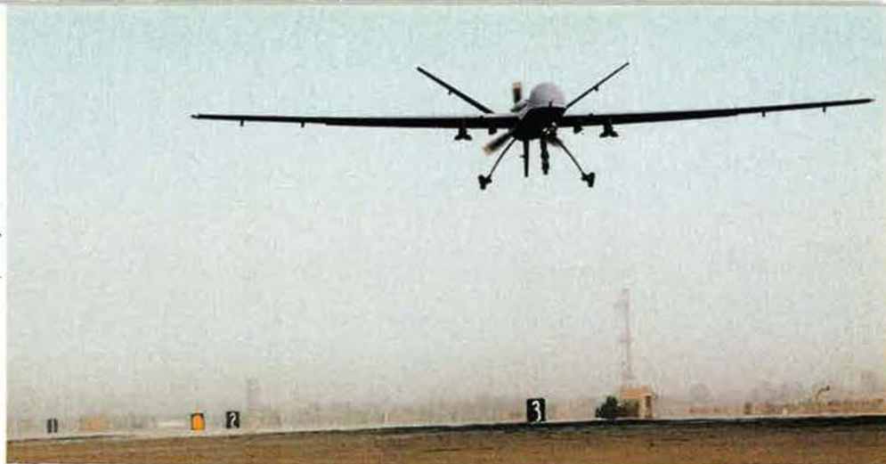
An MQ-9 Reaper takes off on a mission from Joint Base Balad, Iraq. The unmanned aircraft can carry precision weapons, including two 500-pound laser guided bombs.
