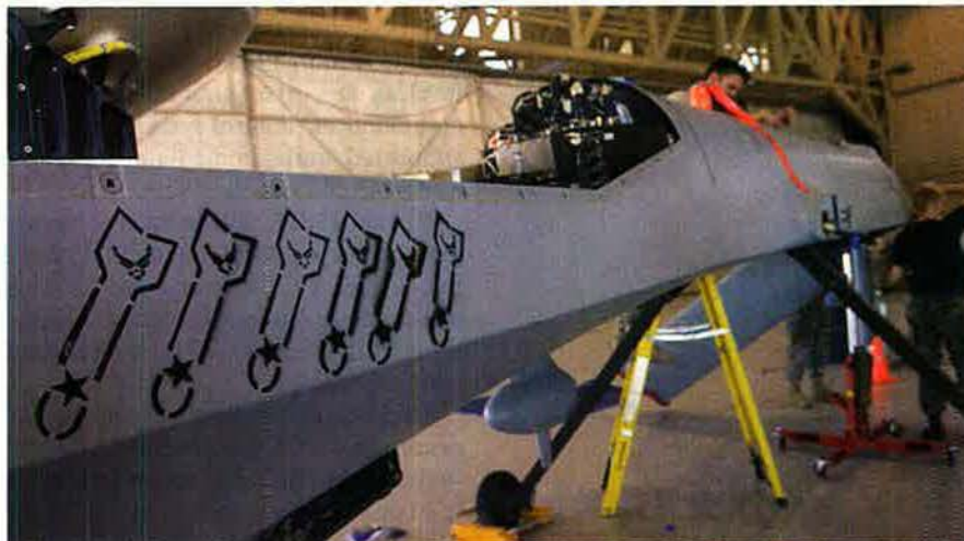
Airmen of the 432nd Aircraft Maintenance Squadron, Creech AFB, Nev., assemble an MQ-1 Predator that has returned from Afghanistan. The markings denote the number of Hellfire missiles it has fired.
