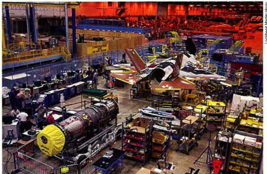
Technicians prepare to install the engine of an F-35 at Lockheed Martin's Fort Worth, Tex., plant.
