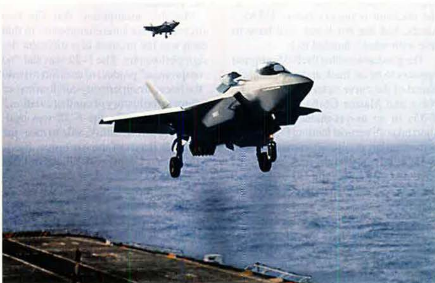
The Marine Corps will fly the short takeoff and vertical landing variant. Illustration depicts an F-35B operating from a carrier.
